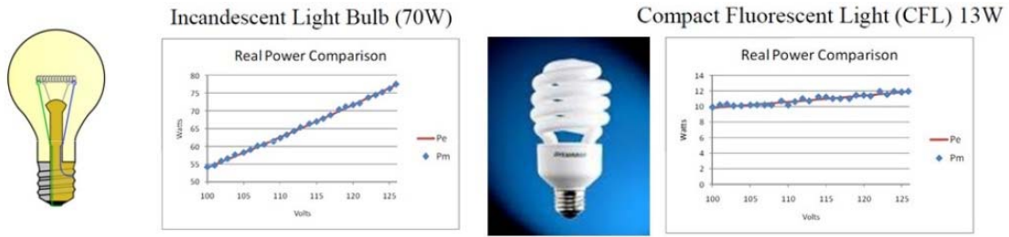
Figure 1. Lamp Type Power-Voltage Profiles from EPRI Report [6]
