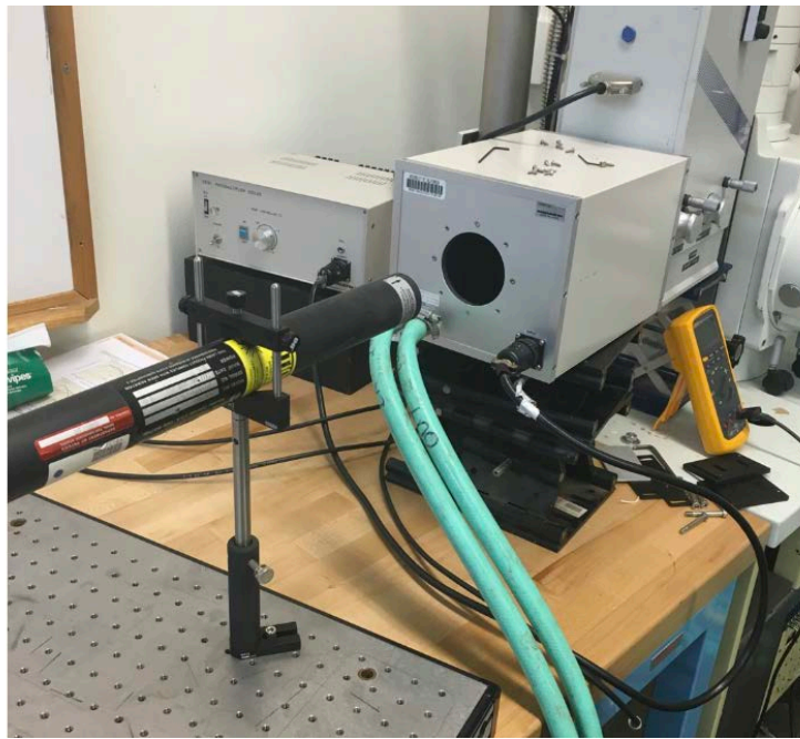
Figure 19. HeNe Laser calibration after posi-drive belt installation.
