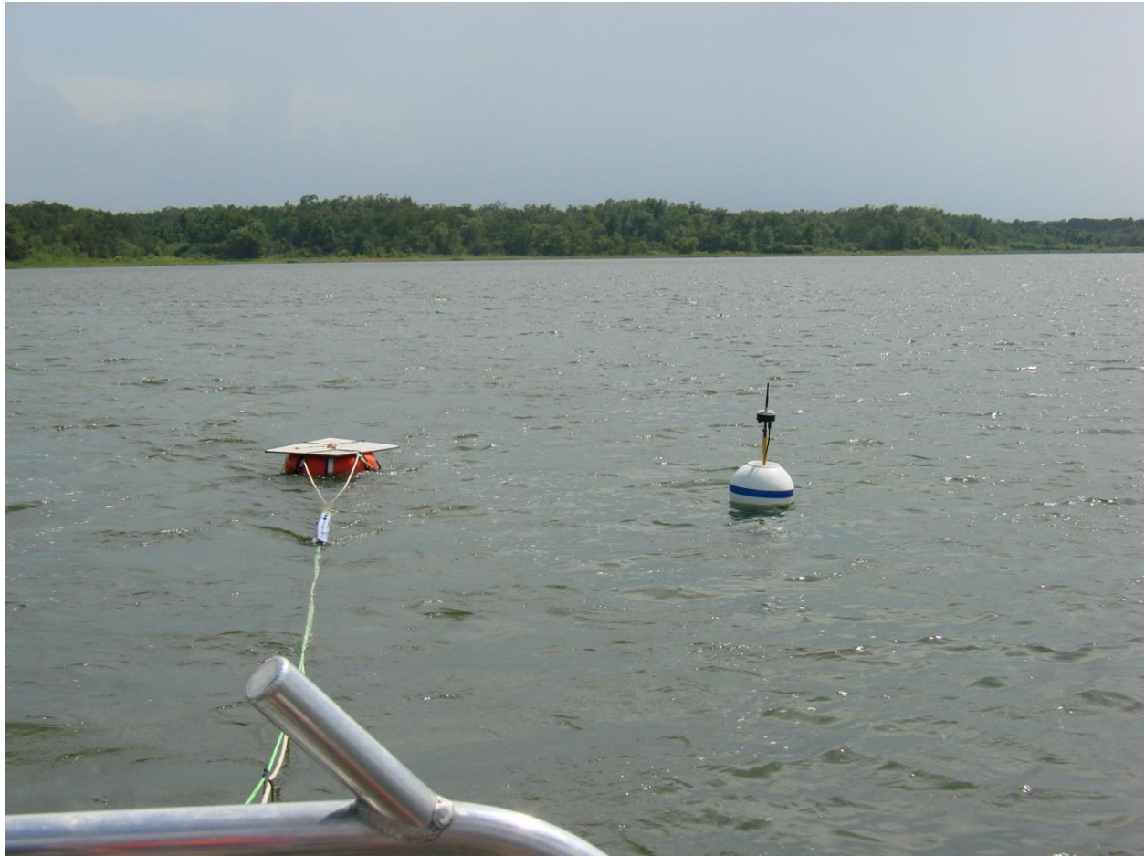
Figure 20: Magnetometer survey under-way
