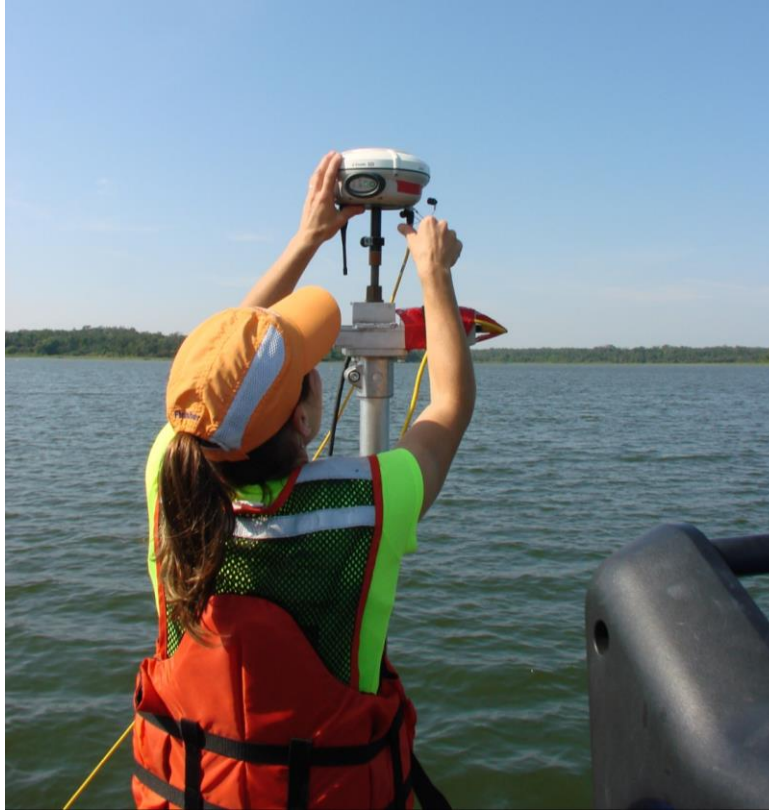
Figure 18: RTK DGPS mounted on top of pinger pole
