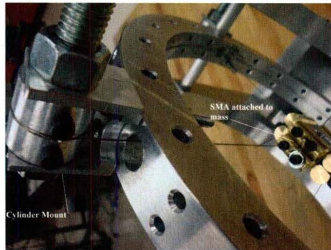
Figure 19 – Cylinder mounts for SMA wires
