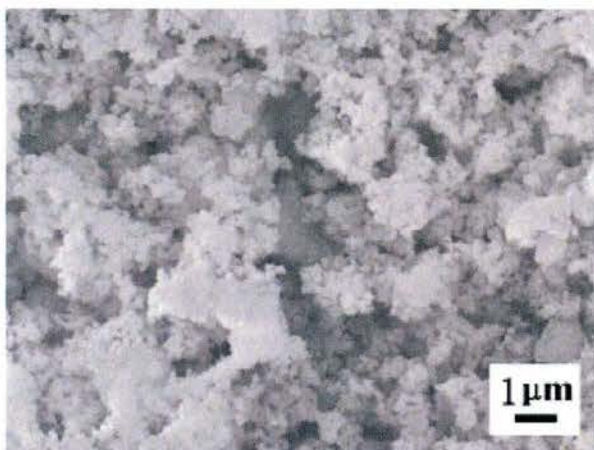
Figure 2: SEM image of the original alumina powder used in this experiment. The alumina particle size is about 0.1 ~ 0.3 μm.
