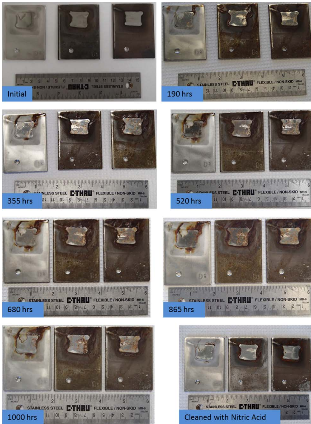
Figure 85. 5002 Group 1 Photographs. As sprayed (left), 950°C/1 hr (center), 800°C/2 hrs (right).
