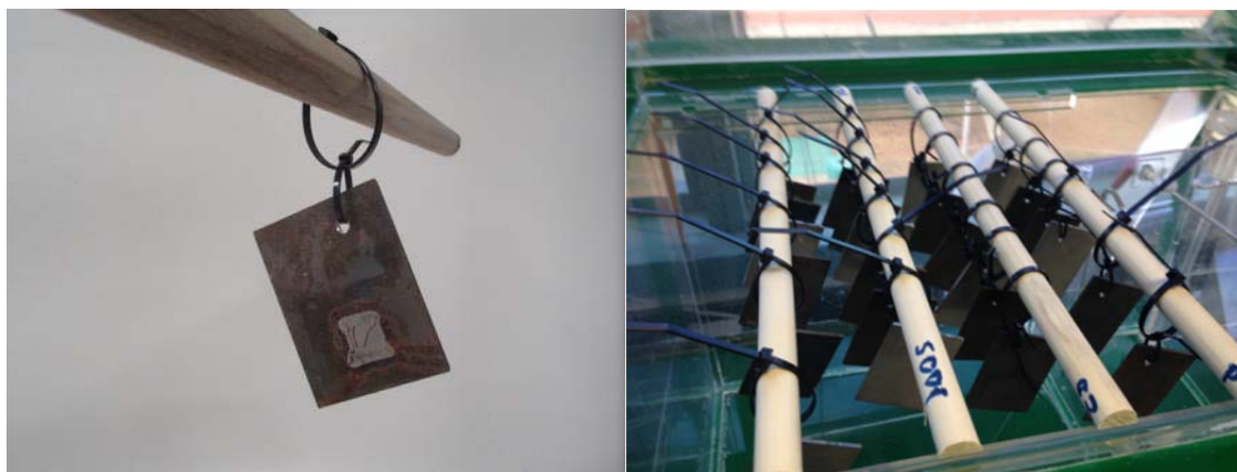
Figure 36. Method of supporting samples in salt fog chamber
