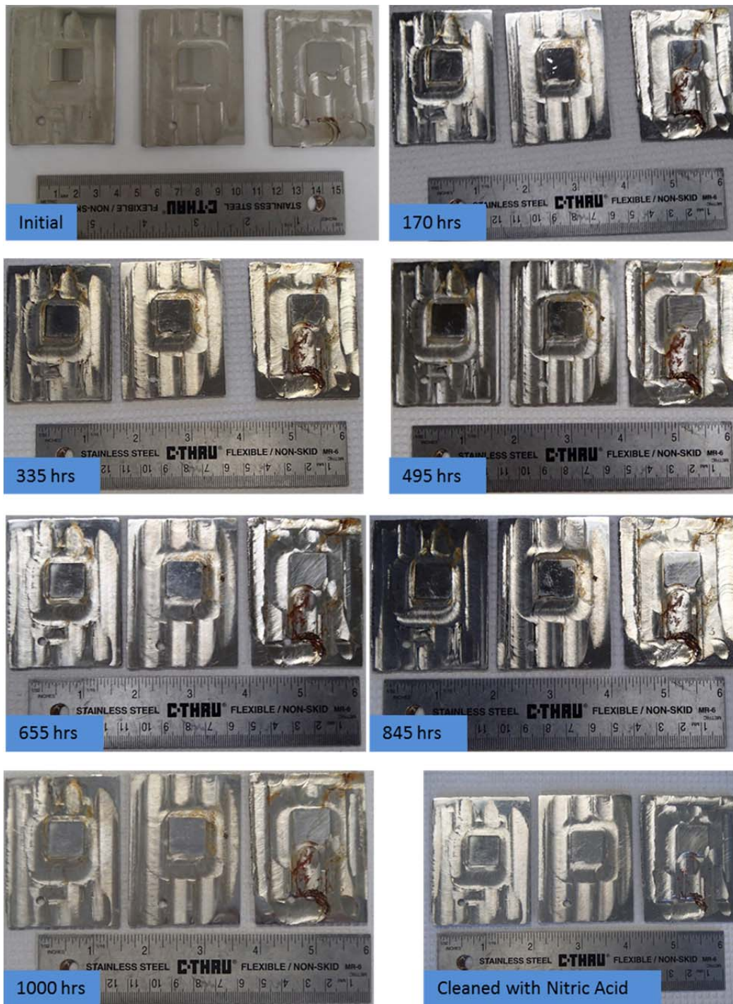
Figure 89. Bare Substrate Photographs. As sprayed (left), 950°C/1 hr (center), 800°C/2 hrs (right).
