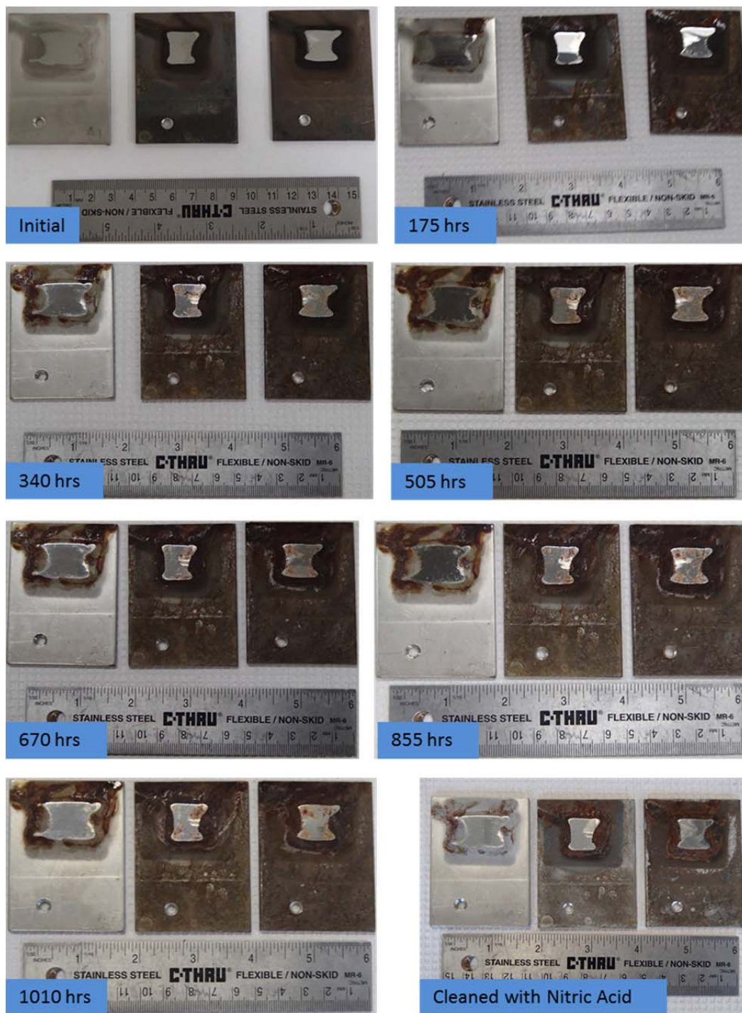
Figure 84. 5001 Group 3 Photographs. As sprayed (left), 950°C/1 hr (center), 800°C/2 hrs (right).
