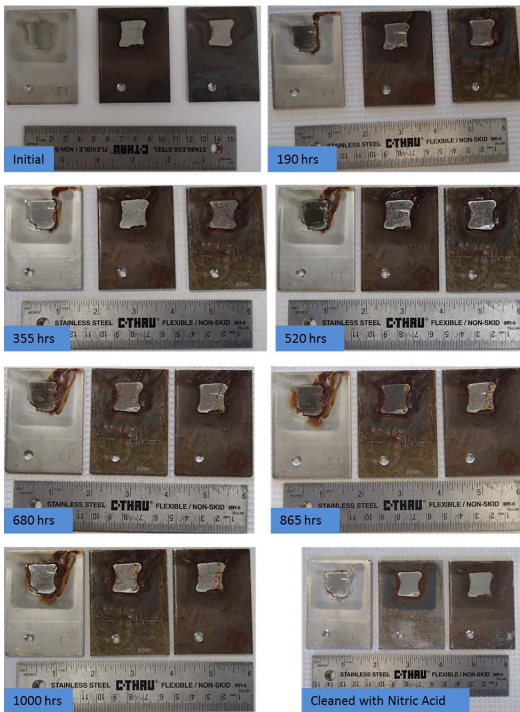
Figure 86. 5002 Group 2 Photographs. As sprayed (left), 950°C/1 hr (center), 800°C/2 hrs (right).
