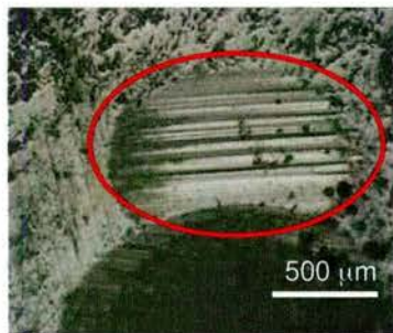
Fig. 16 Micrograph of surface after testing of specimen without metal phases
