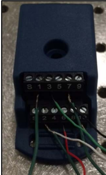
Figure 79. Load Cell Wire Leads into NI-9949 Terminal Screw Adaptor.
