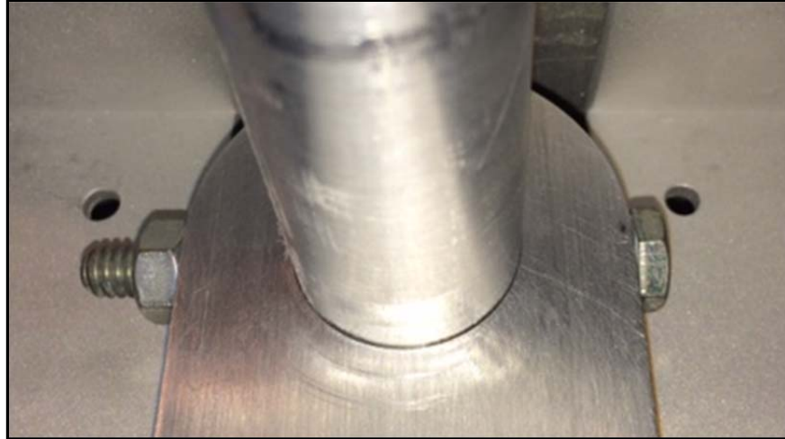
Figure 35. Attachment Point for Rotating Rod and Pendulum Arm.
