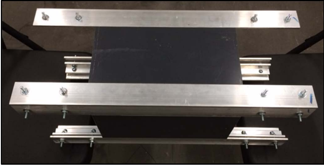
Figure 10. Assembled Composite Form (side).
