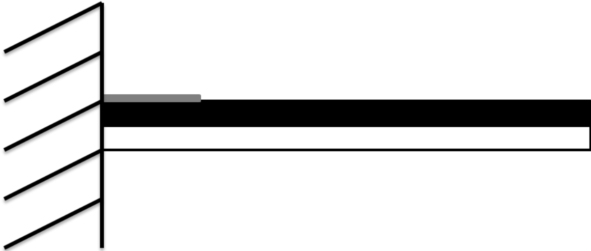
Figure 27. Cantilever Beam with Piezoelectric Base
