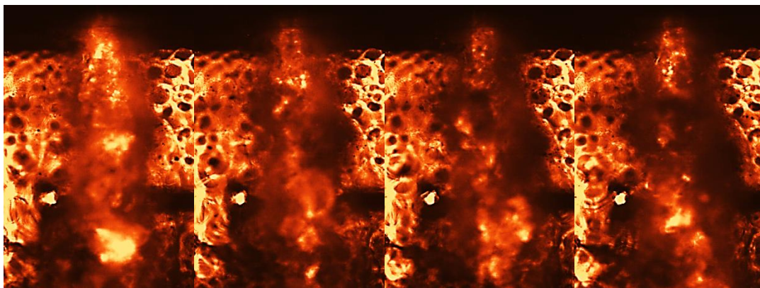
Figure 7 – Time series of an instantaneous shadowgraph images. A dark soot cloud can be seen obstructing the view to the center core.
