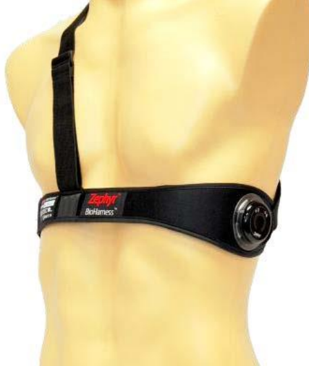
Figure 28. BH3 inserted into chest strap and affixed on a mannequin
