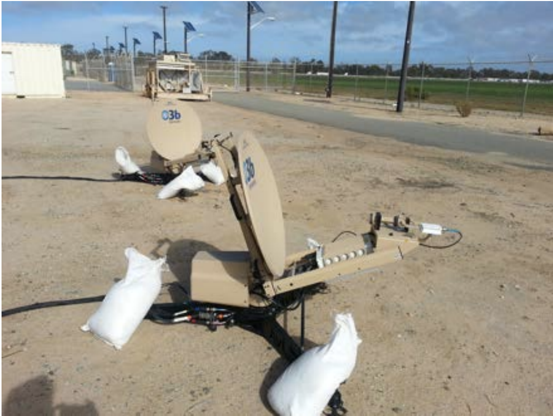
Figure 23. Tracking Fly Away Antenna System Terminals
