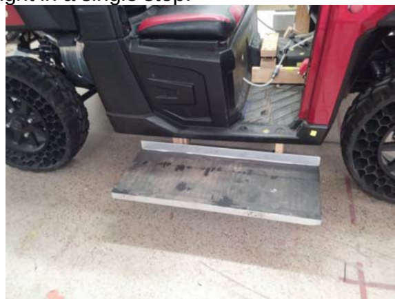
Figure 47. Picture of the vehicle with the step addition. The step provided an intermediate platform so that the robot did not have to step down the full vehicle height in a single step.
