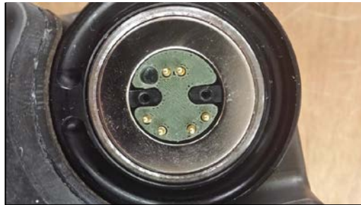
Figure 28. Modified routing hole of iRobot hand for reduced tendon breakage.
