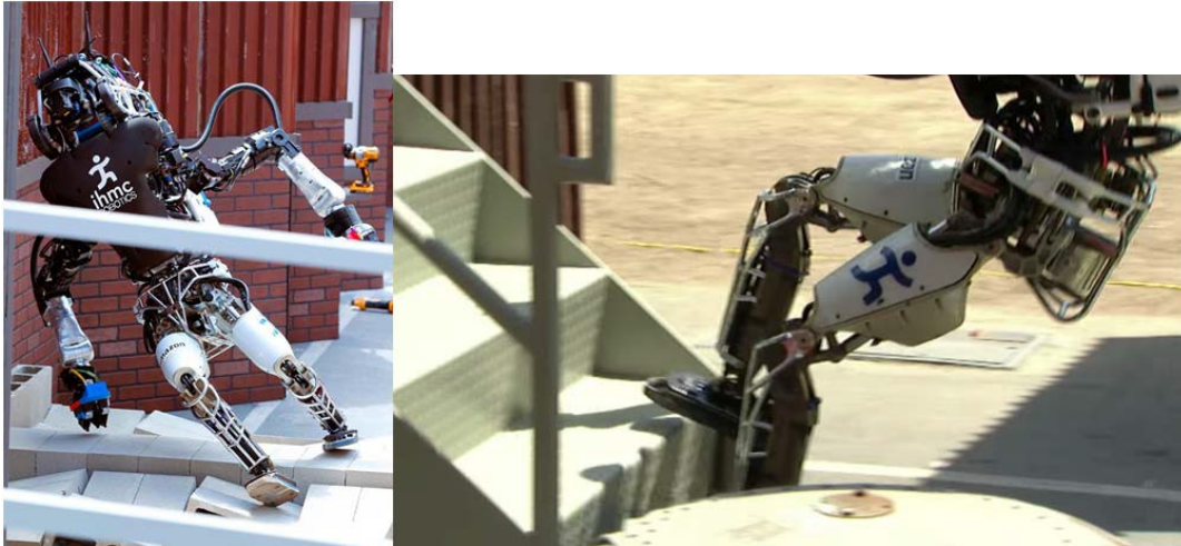
Figure 42. Team IHMC fell two times during the first day of the DRC finals. The fall on cinder blocks was due to taking an aggressive step without selecting a walking configuration used for aggressive steps. The fall on the stairs was due to a combination of rushing since we were low on time, a programming bug, and body oscillations that we think were a result of falling on the cinder blocks. After day one, we made corrections for both falls and were able to successfully complete all eight tasks on day two.
