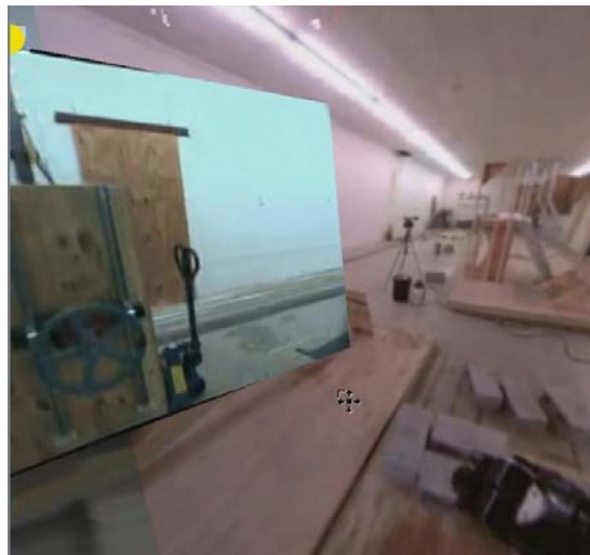
Figure 33. Images from head and chest cameras fused together into the first person viewport. The higher resolution rectangle is the normal camera and the rest of the image is from the fisheye camera. This gives the operator the illusion of looking to the right even though the robot cannot yaw its head.
