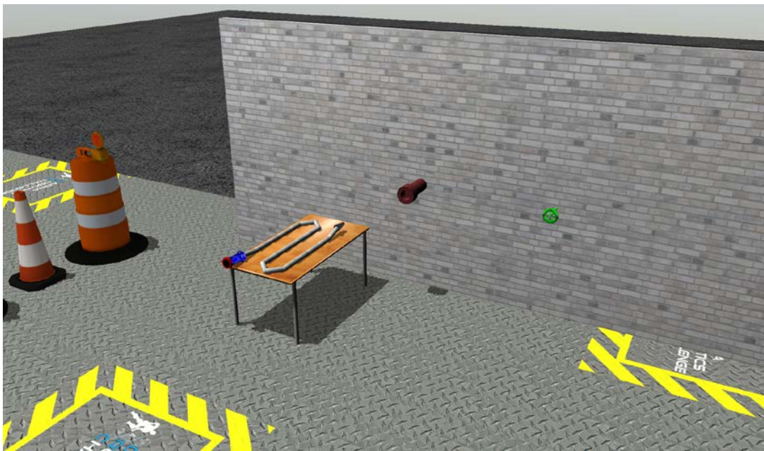
Figure 21. Custom manipulation task with a larger and more massive hose connector, lower table, valve and standpipe placement reversed, and smaller valve with higher damping parameter.
