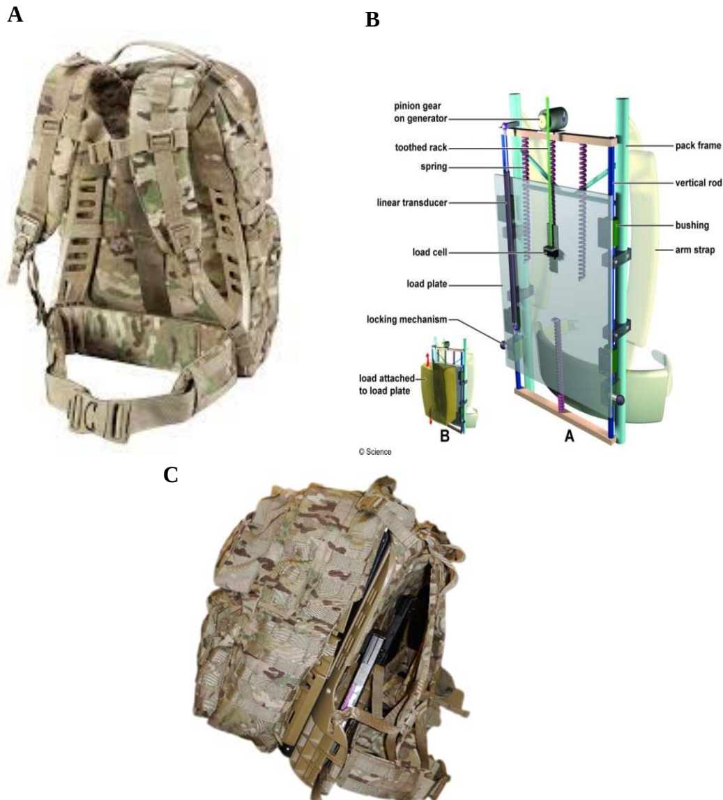
Figure 1: (A) MOLLE medium rucksack. (B) Schematic of the load plate and frame for the prototype electricity generating pack from Lightning Packs, LLC. (C) LP medium rucksack.
