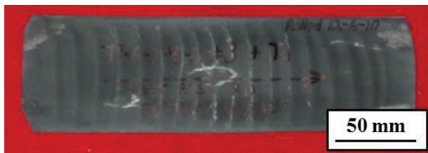
Figure 7. Photograph of a Ti-6Al-2Sn-4Zr-2Mo-0.1Si foil which was hot packed rolled.
