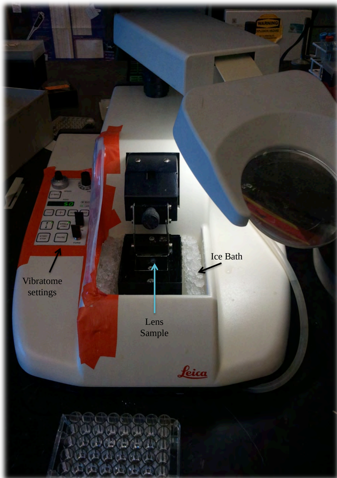
Figure 3.3: Leica Vibratome used to section internal lens fiber cell samples (in MCDB facility)
