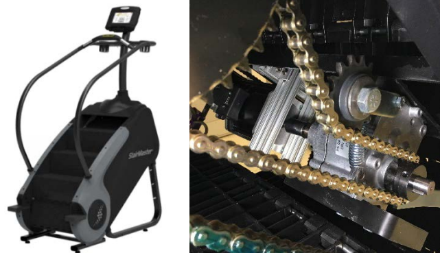
Figure 7: Stair Descent Machine. We have replaced the resistive alternator with a powered motor for reverse direction operation.
