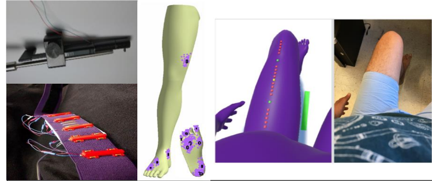
Vibrotactor single stimulator (left, top) and worn array (left, bottom). Vibrotactile sensory feedback can deliver sensation of forces and foot events to the lower extremity amputee. Users having targeted reinnervation feel these sensations as if they are originating at the absent limb. Participants indicate where they felt sensations (middle). Sensory characterization is also performed by providing simultaneous visual and tactile sensation (right).
