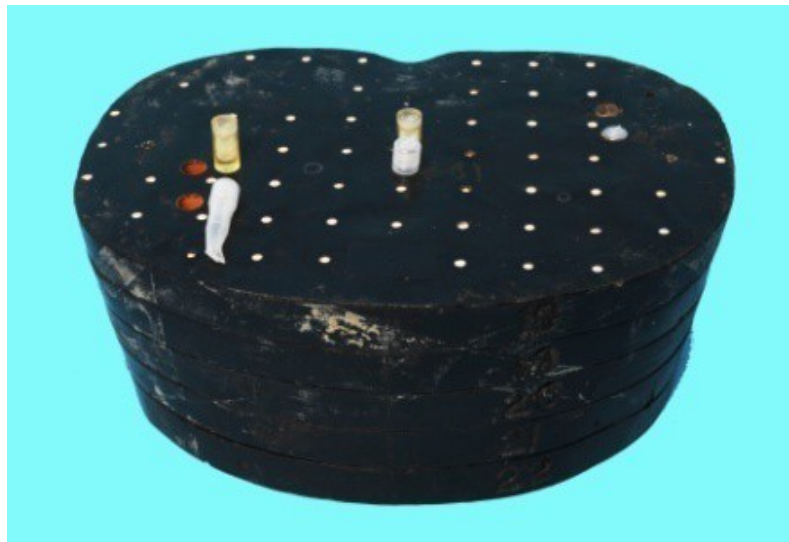
Figure 2-2B For each cobalt-60 exposure, dosimetry vials and sample vials are present. For dosimetry exposures the dosimetry vials contain alanine pellets and the sample vials are empty. For exposures with virus the dosimetry vials are empty
