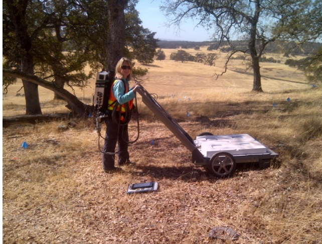
Figure 2-6. TEMTADS Man-Portable 2x2 Cart Sensor Platform
