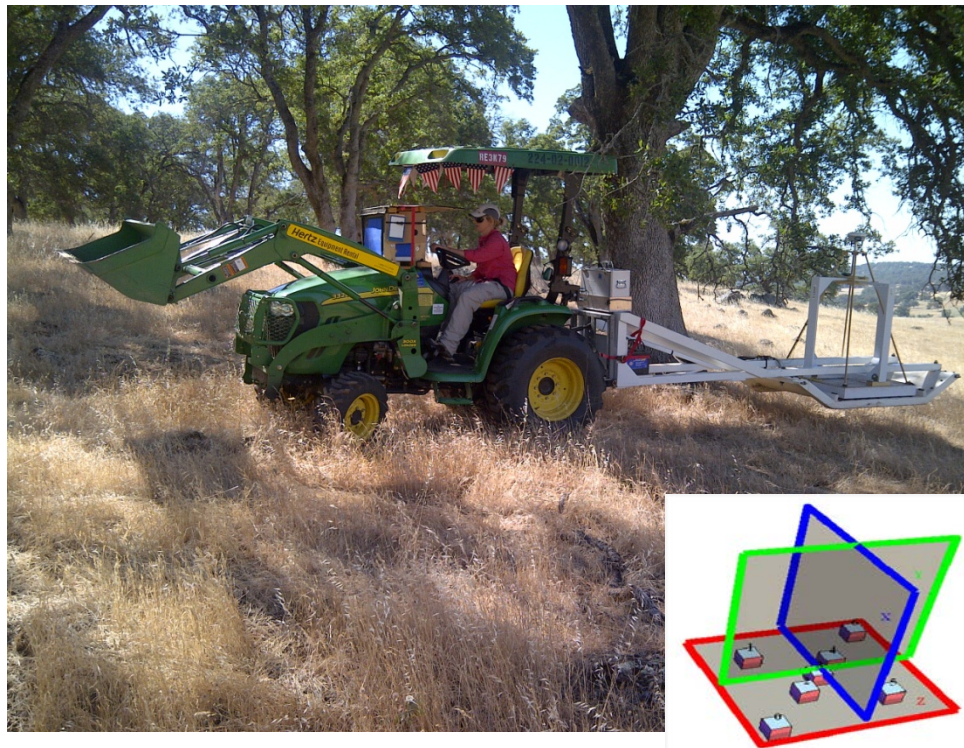
Figure 2-2. Antenna Array and Typical Deployment of the MetalMapper System
