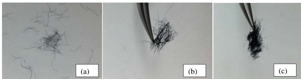
Fig. 96 After thermal-oxidation up to 220 °C at a heating rate of 0.4 °C/min: a) with prior UV treatment of fibers; b) control fibers; c) as-spun fibers
