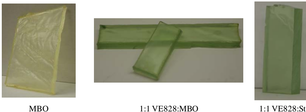
Fig. 115 MBO (left), 1:1 VE828:MBO (middle), and 1:1 VE828:St (right) thermosets
