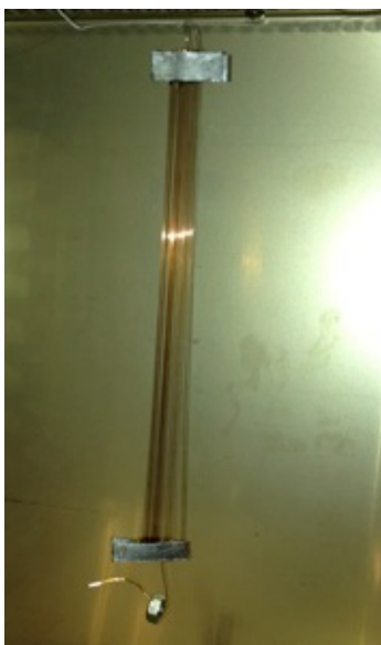
Fig. 88 Fibers stabilized with constant load displayed extension during stabilization
