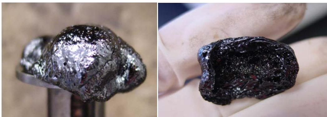
Fig. 57 Foamed soda lignin after heating to 250 °C
