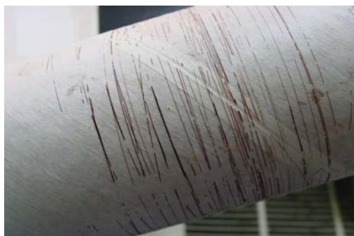
Fig. 78 Photograph showing sticking of Ace-SKL to the roll surface due to insufficient evaporation of acetone
