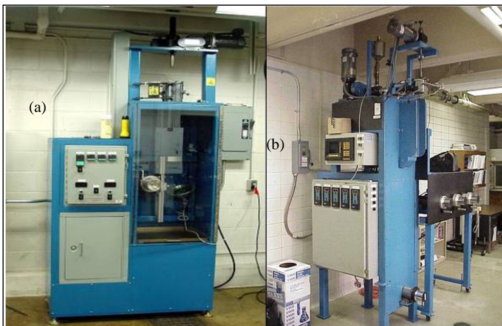
Fig. 21 a) Batch-spinning unit for samples up to 100 g and b) continuous fiber-spinning unit for large-scale laboratory production of fibers at rates up to 5 kg/day
