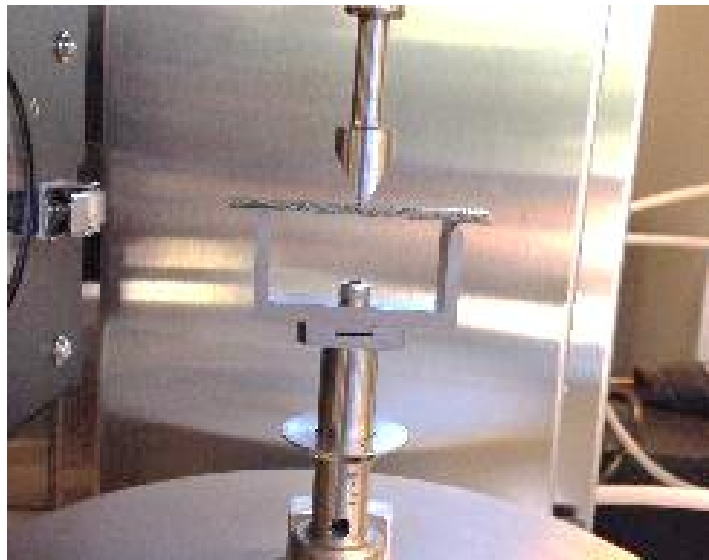
Fig. 198 Three-point bending test of T-300-based carbon fiber composite
