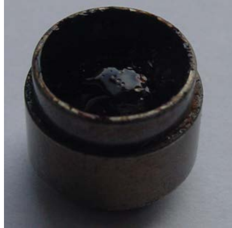
Fig. 51 A consolidated melt resulting from softening point test on Ace-SKL (ball removed)
