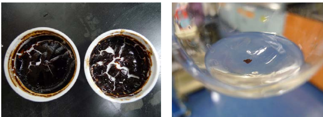
Fig. 68 Left: Film chips made from methacrylated SKL. Right: Film chips of methacrylated SKL tested with acetone.
