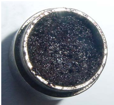
Fig. 50 Unmelted, foamy residue resulting from softening point test of pure SKL (ball removed)
