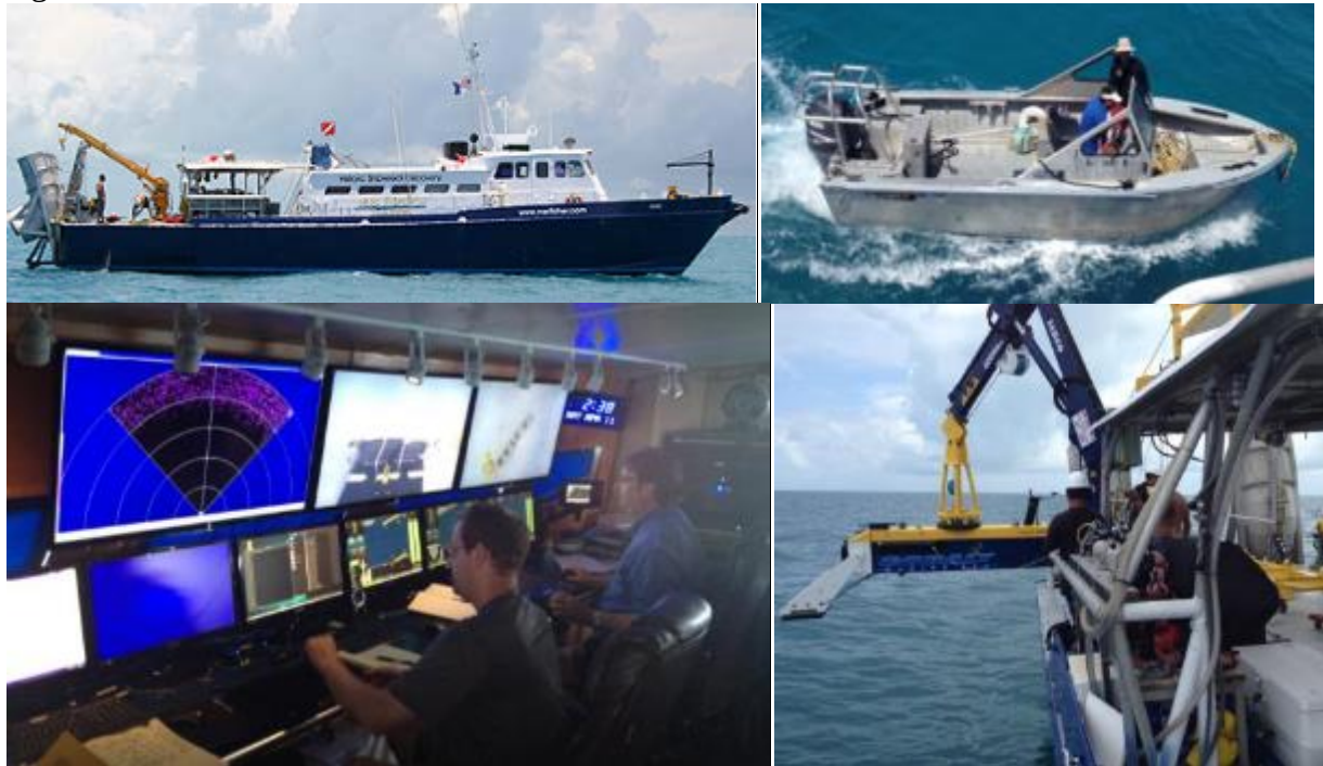
Figure 29. Top Left: R/V Dare - a 84-foot modified dive salvage and crew boat to which the HAUV-100 is currently dedicated. Top Right: The 17-foot Boston Whaler tender and anchor vessel that accompanies the Dare. Bottom Left: Maine control room and ROV operations monitors. Bottom Right: Stearn ROV deployment.
