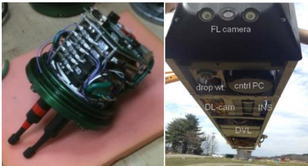
Figure 4. Left: Photograph of the inside of the subsea NCS pressure vessel. This processing and inertial core sensing unit works in conjunction with external aiding sensors such as DVL, USBL, altimeters, and depth sensors. Right: The NCS pressure vessel installed on the Dolores HAUV platform.
