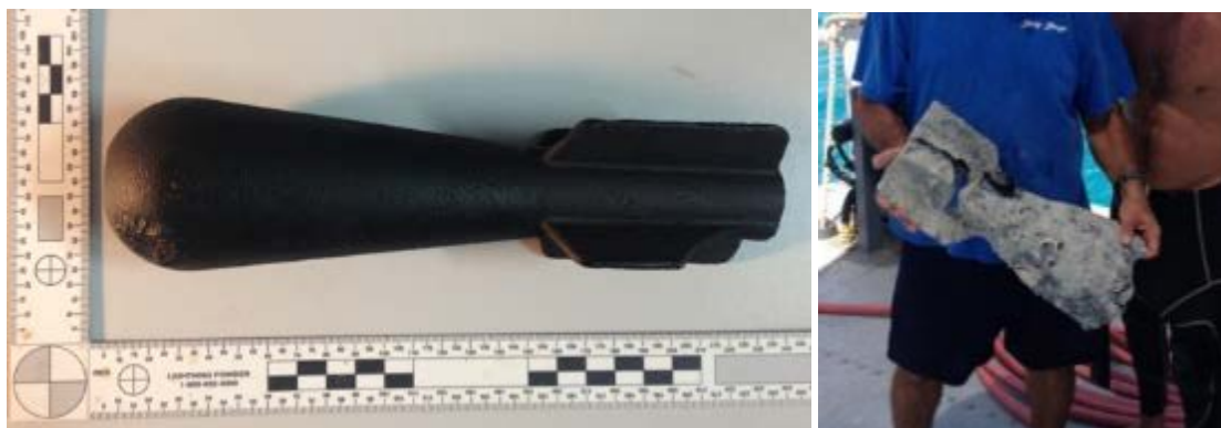
Figure 43. Photographs of AN-MK 5 Mod 1 practice bomb uncovered during salvage operations near our proposed site area. Left: Dummy bomb test item; Right: Tail section of dummy bomb detected with the ROV-EM system and recovered from the sea bottom.
