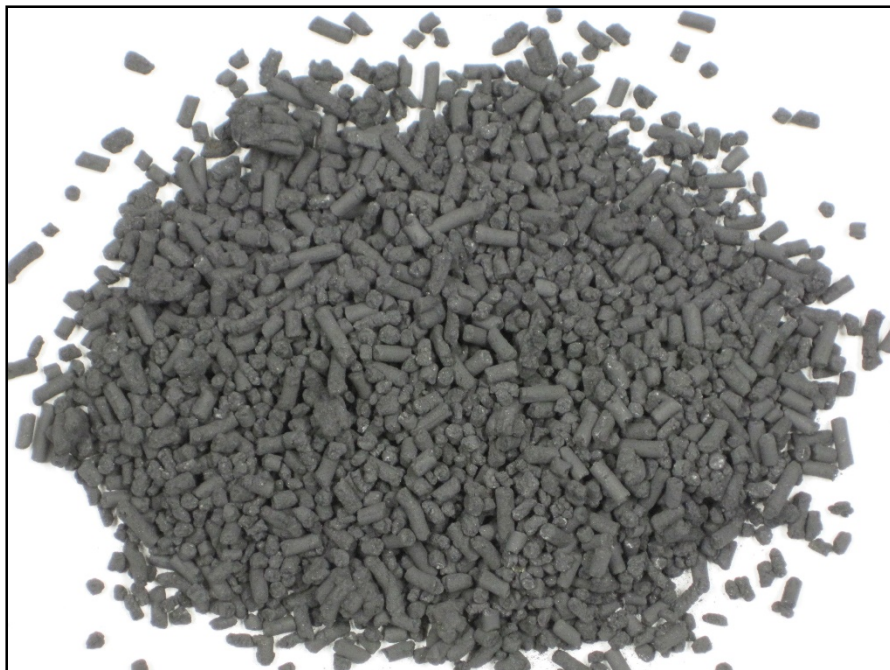
Figure 1. SediMite ® pellets containing powdered activated carbon (PAC). The pellet is an agglomerate that includes the treatment agent (PAC), a weighting agent (sand), and a binding agent. Once wetted, the pellet releases the fine-particle-size treatment agent to sediments or wetland soils. SediMite ® can include PAC or any other treatment agent or mixture of agents that can benefit from pelletized delivery.
