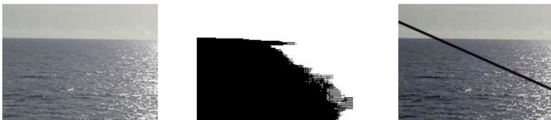
Figure 4. Horizon Detection with Supervised Learning. Source [14].
