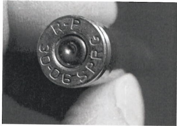
Figure 4: DDNP-based KVB-7E primer which produced a misfire in a 30-06 test load. The crater suggests the misfire was not due to a light primer strike. The other nine 30-06 test loads with this primer demonstrated a perceptible delay in ignition.
