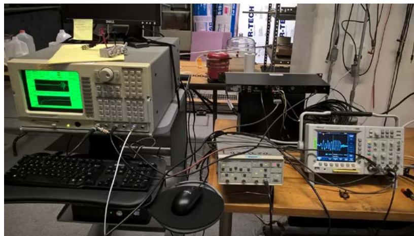
Figure 89. Setup for Measure the Reciprocity Calibration in Water.
