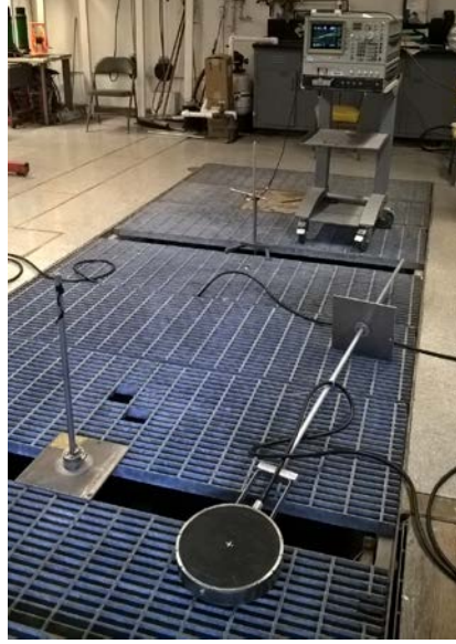
Figure 90. Reciprocity Calibration of F 33 and Planar Magnetic Transducers.
