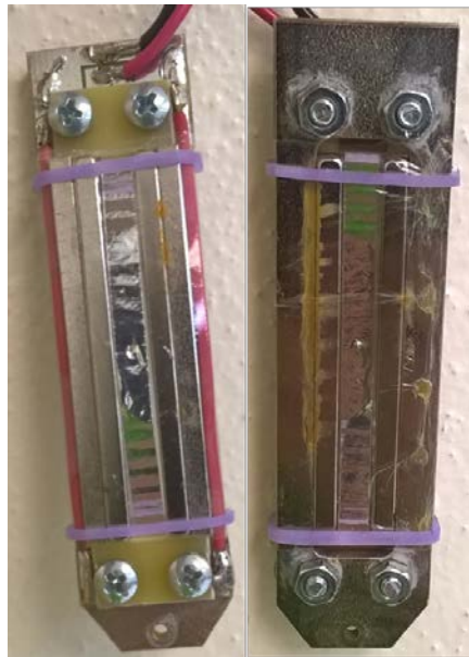
Figure 62. True Ribbon Transducer Damaged.
