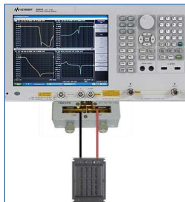
Figure 20. Block Diagram to Measure the Complex Impedance.
