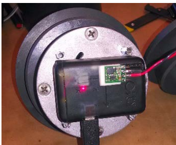
Figure 8. IMU mounted on the endcap of the pressure case inside a surrogate UXO
