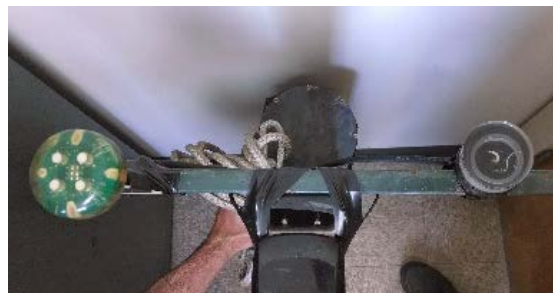
Figure 9. USBL array (left) and interrogation transponder (right)
