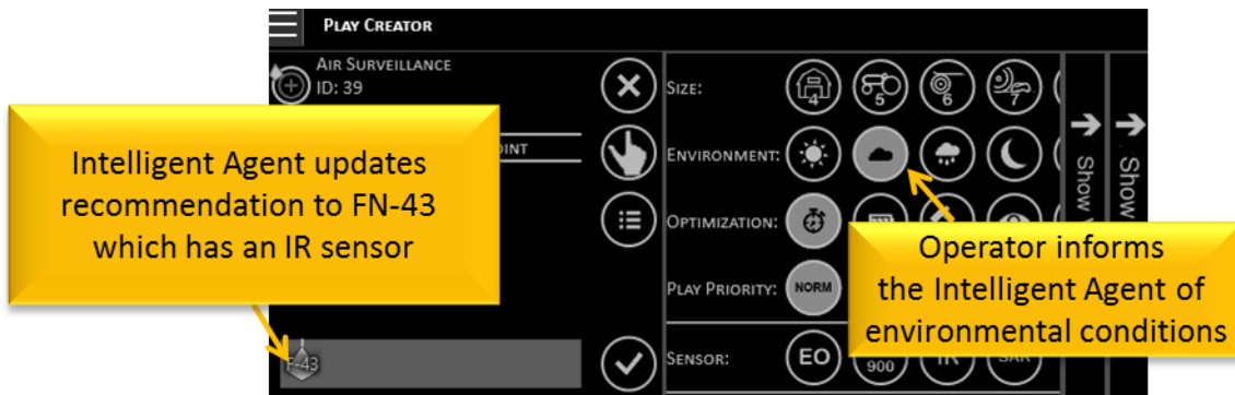
Figure 10. Operator providing information to the Intelligent Agent including environmental conditions (the cloud icon is selected), optimization preference (the stopwatch icon is selected), and priority (normal is selected). The Intelligent Agent has recommended FN-43 (which has an IR sensor) based on these operator inputs.
