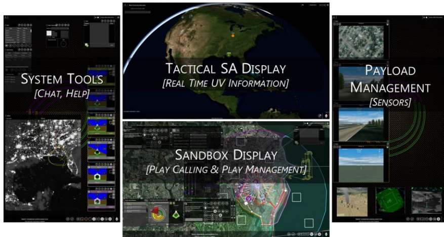
Figure 3. A screenshot of IMPACT’s test bed interface, with the tactical situation awareness display on the top monitor, the payload management display on the right monitor, the sandbox (planning area) on the bottom monitor, and system tools on the left monitor.
