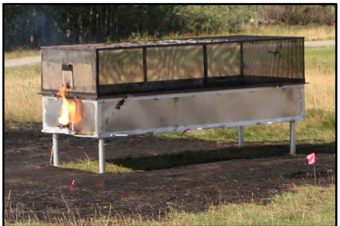
Figure 6. Initiating propellant in slider.
