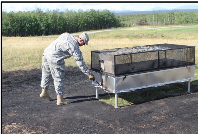
Figure 6. Initiating propellant in slider.
