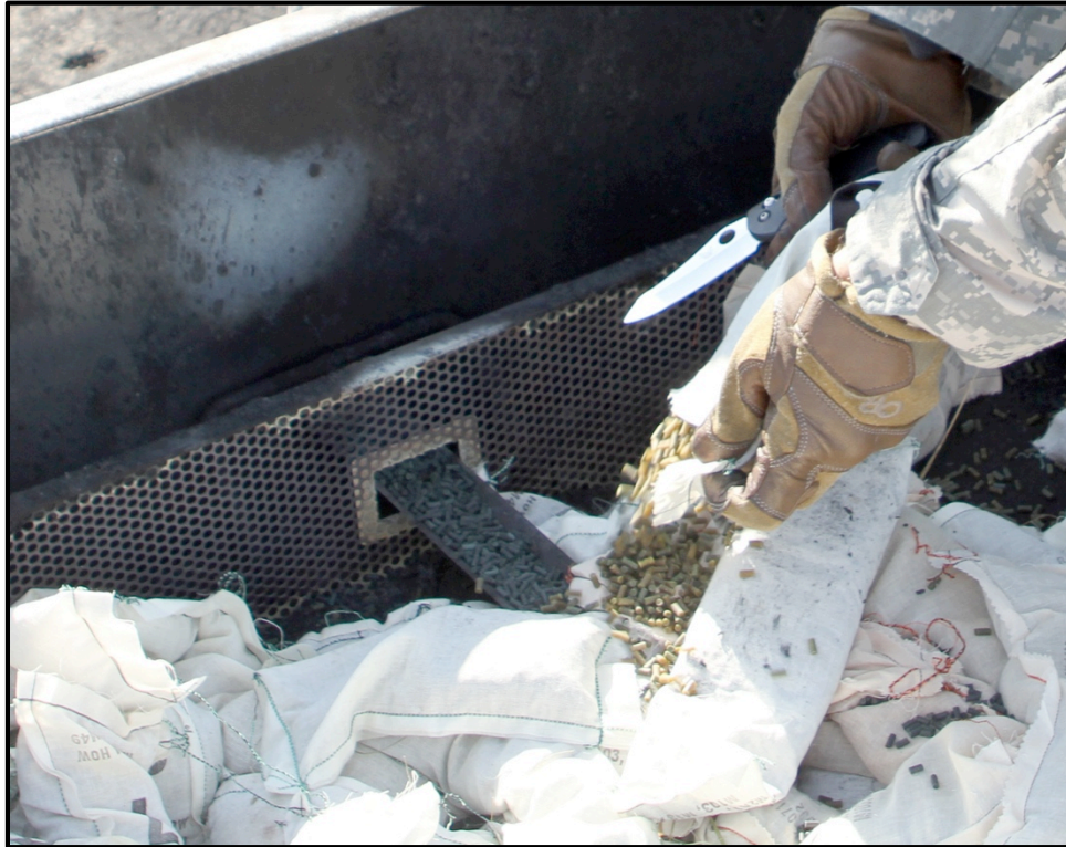
Figure 5. Placing propellant grains at end of slider to initiate burn.
