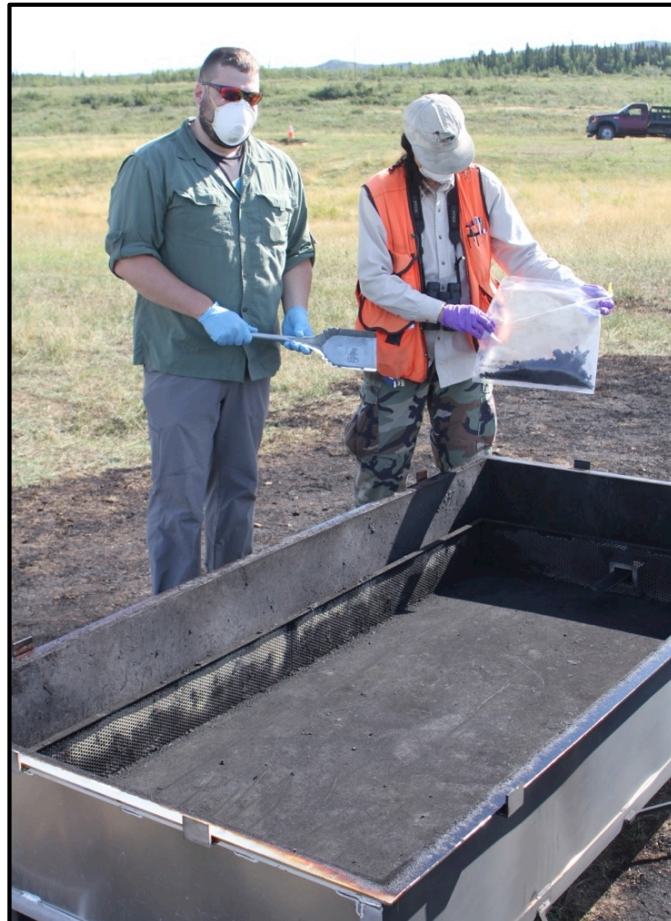
Figure 8: Residues collected from false bottom of pan following completion of testing.
