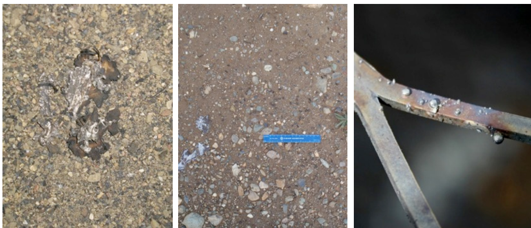
Figure 6. Lead from the decoppering foil in propellant charge following burn events. Lead foil remnants with a partially burned charge bag on soil near a fixed burn pan, lead foil with propellant grains on the ground adjacent to a fixed burn pan, and fine lead particles on the 3-mm steel open-mesh grate of a prototype portable burn pan following a 120-kg test burn.
