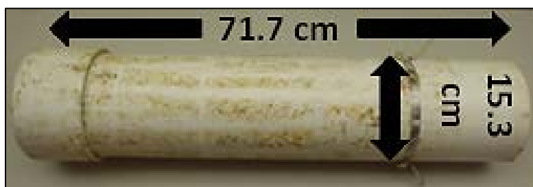
Figure 5-15. Sediment trap used for quantification of sediment particles and contaminants of concern over the sediment remedial cap located by Pier 7 at the PSNS&IMF.
