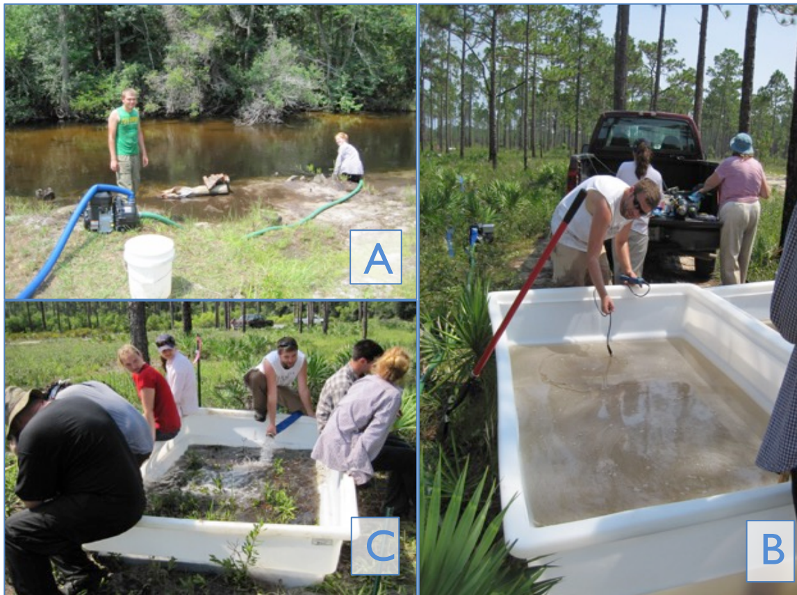
Figure 2. Steps in the experimental storm surge treatment. In panel A, ~757 L of water is pumped from the East Bay River into a holding tank. The holding tank is shown in panel B; here, the salinity is measured and Instant Ocean™ marine salt is added and mixed to achieve 27 ppt. In panel C, all water from the holding tank is being pumped into one of the vegetation plots.
