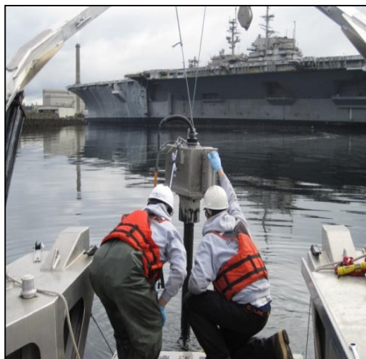
Figure 3-5. Core Sample Locations at Bremerton Naval Complex (top); Core Collection Using a Vibracore Mounted on a Vessel (bottom)
