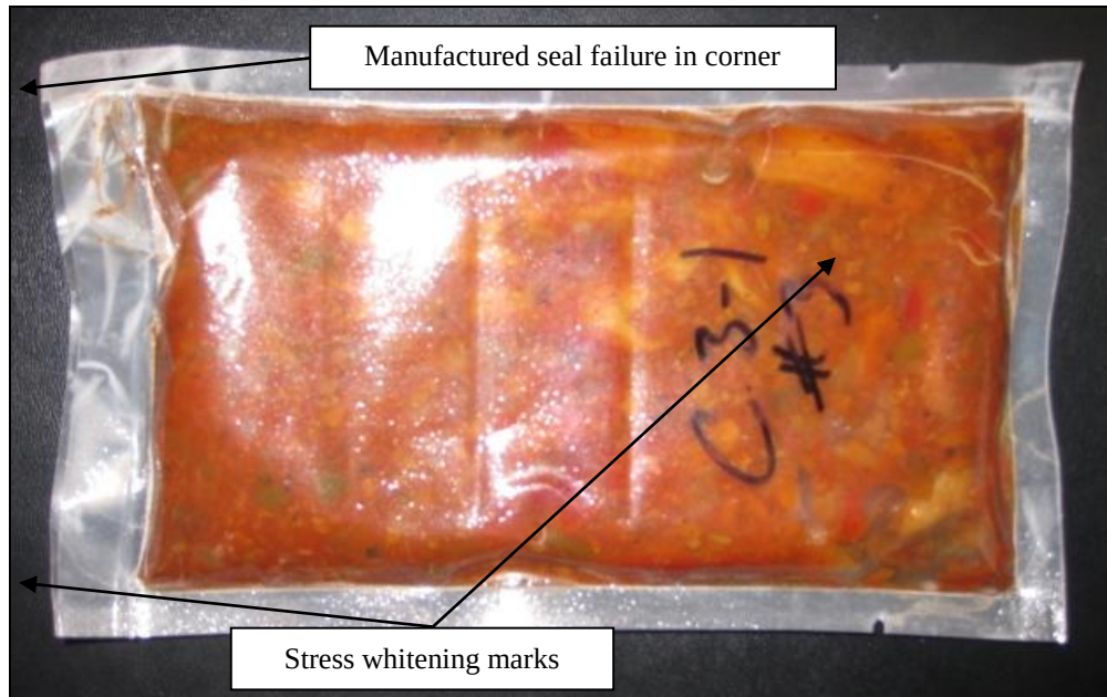
Figure 74. Stress Whitening and Failure of Manufactured Seal Resulting in Product Exposure (C GL/KN 3-1-3)
