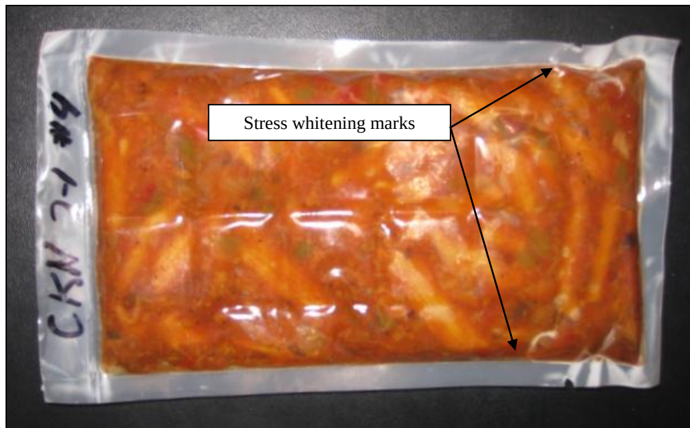
Figure 75. Stress Whitening of Prototype Retort Pouch (C KN 2-1-1)
