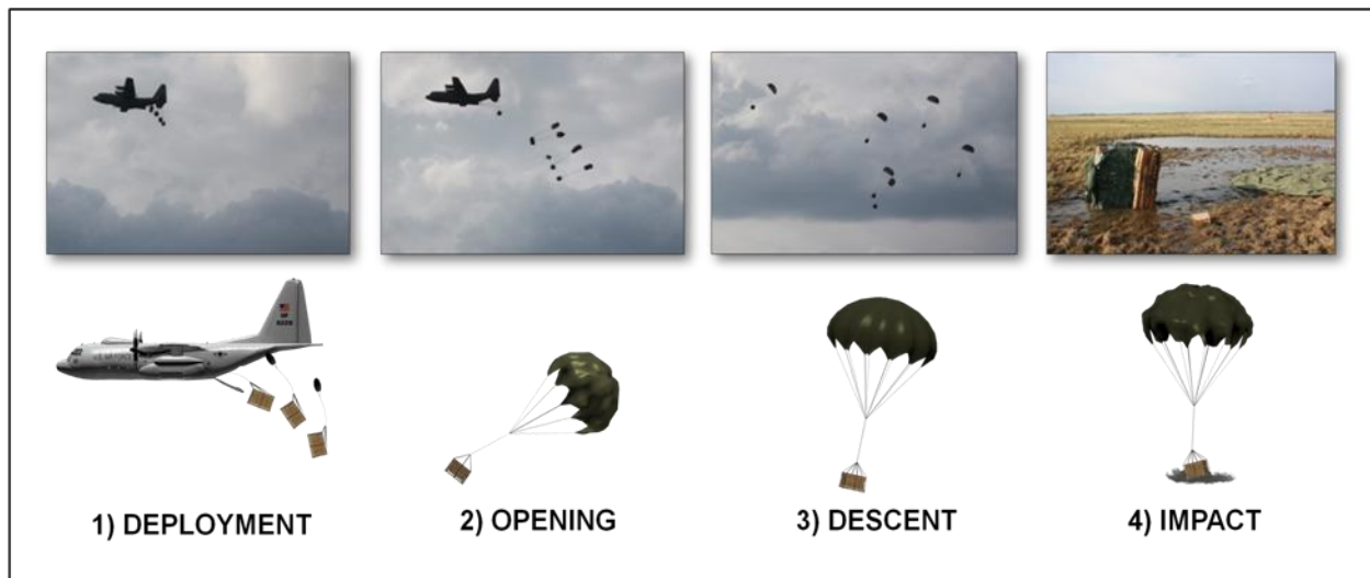
Figure 16. Drop Sequence for Aerial Delivery (High Velocity Drop Sequence - 11/15/2010)
