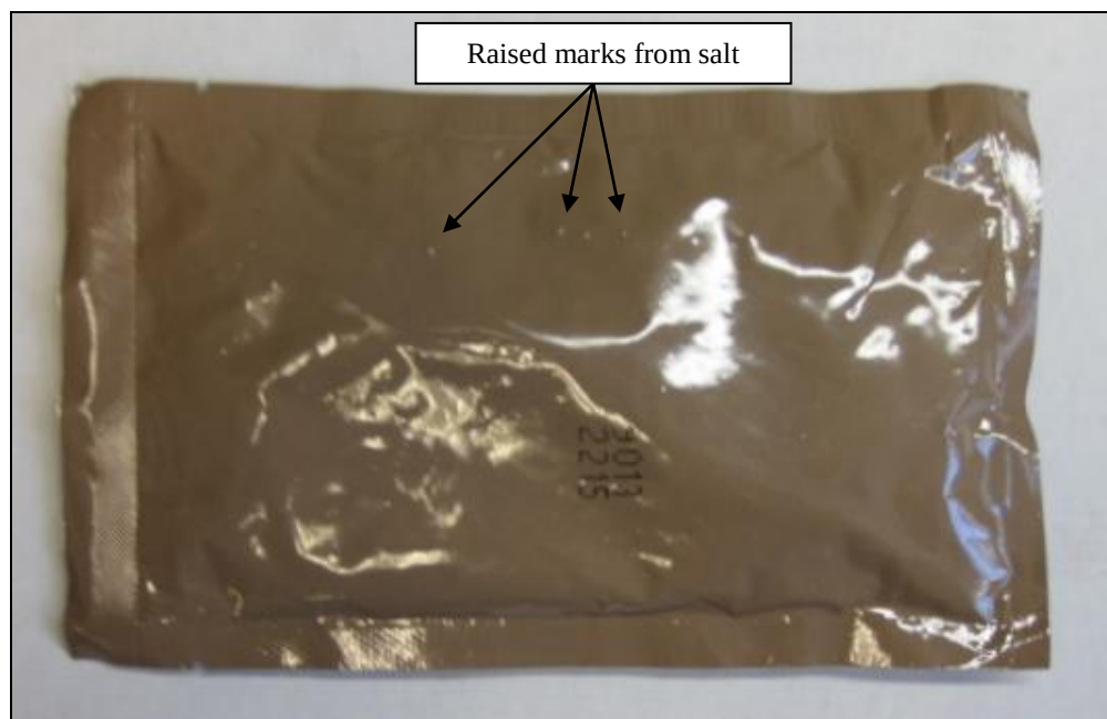
Figure 73. Damage Marks from Salted Pretzels (Control Pretzel Pouch).
