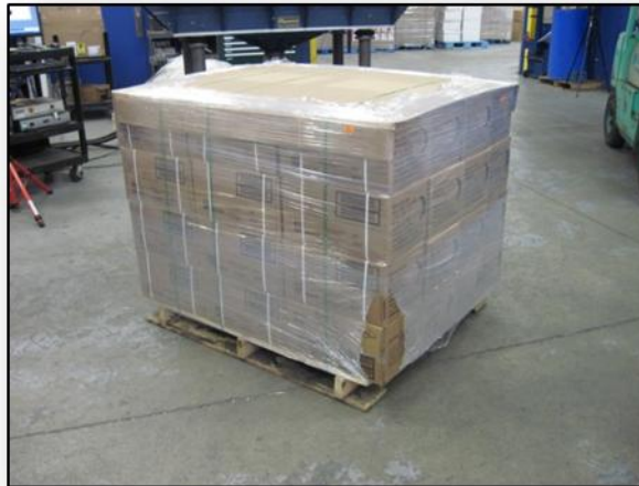
Figure 45. Damaged Stretch Wrap Upon Arrival (Each unit was rewrapped prior to testing).
