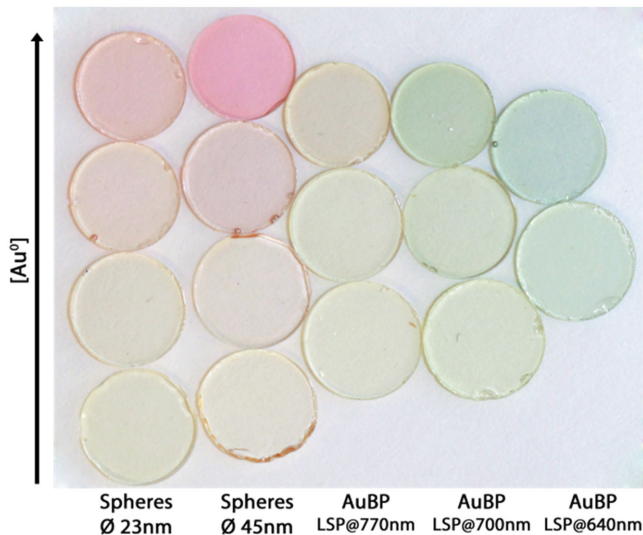
Figure 5. Monoliths after optical polishing. The material with the highest concentration of AuBP (LSP@640 nm) is missing in the picture.
