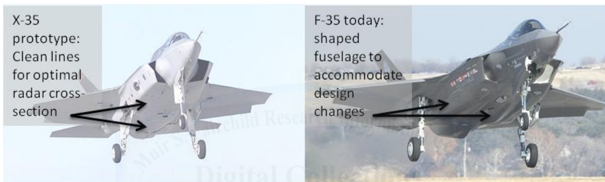
Figure 2. Images showing the design changes in the F-35 that Dr. Kopp argues lead to less-than-optimal stealth capability. (Adapted from "Assessing Joint Strike Fighter Defence Penetration Capabilities.")
