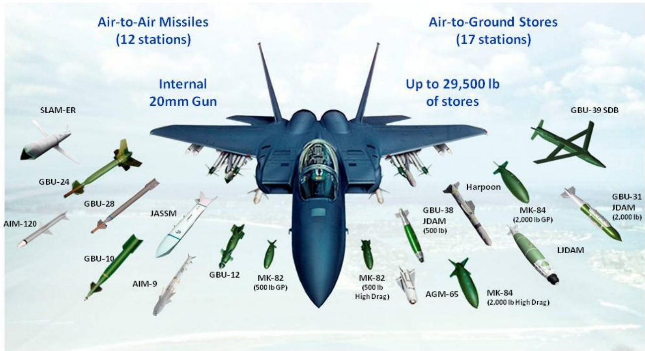
Figure 9. Weapons Carriage capability of F-15SE “Silent Eagle”. (Reprinted from a 2010 Boeing Presentation, “Silent Eagle Overview.”)
