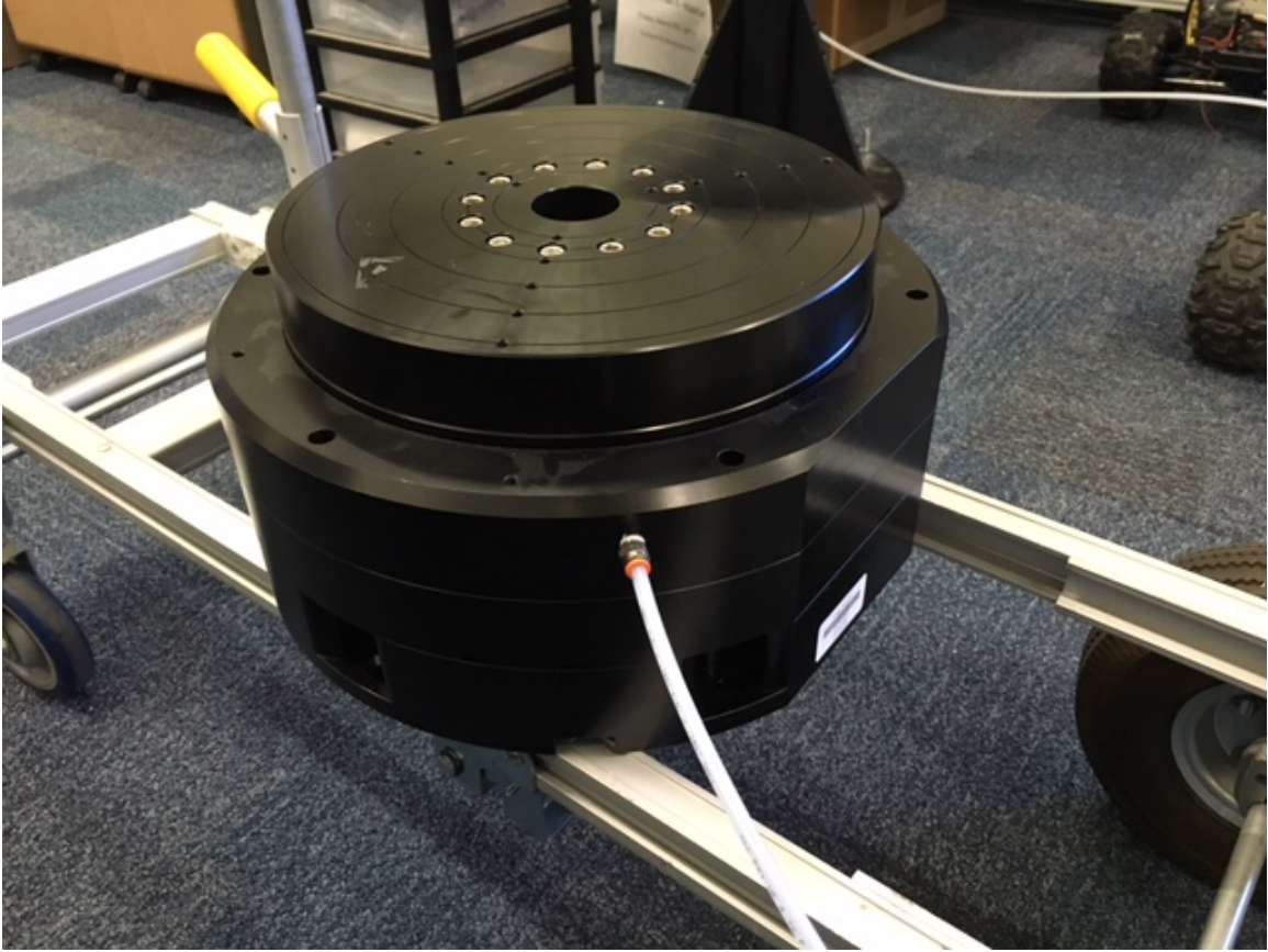
Figure 12. Single Axis Air-Bearing Test Set
