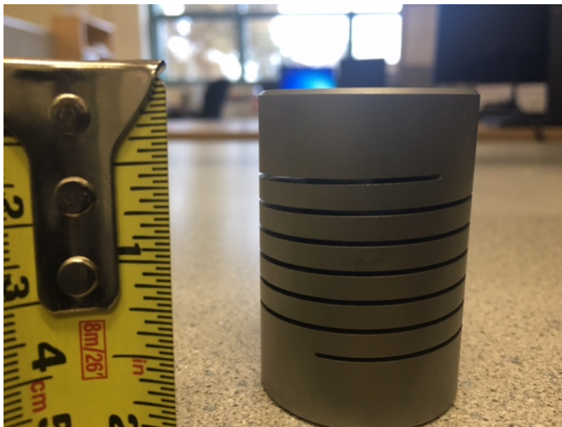
Figure 38. Side View of Helical Machined Spring Manufactured for Test Bed
