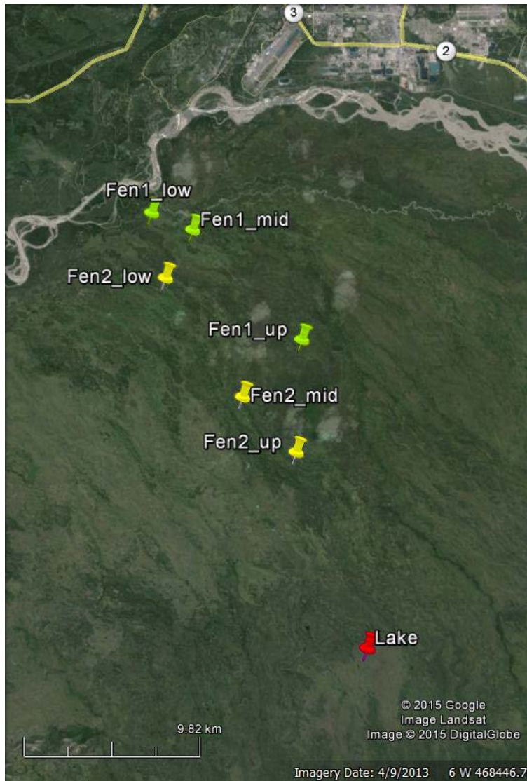
Figure 9. Locations of the groundwater monitoring wells in the two parallel fen systems (Fen 1 and 2) and the lake. Fen 1 and Fen 2 are separate fen systems but both are believed to be linked to the lake as the initial surface water source. Wells were installed at every marker location.
