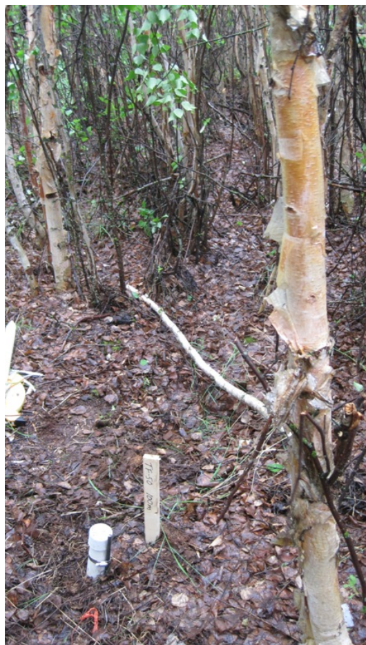
Figure 36. A photo of the thermistor installation from transect location 100 meters at the 1988 fire scar site.
