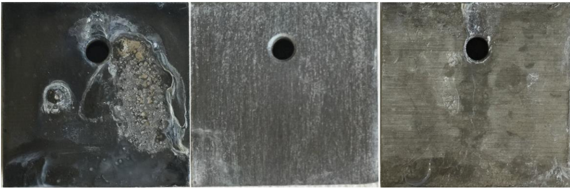
Figure 45. Corrosion Test Week 5, Left Superhydrophobic, Middle Superhydrophilic, Right Untreated.
