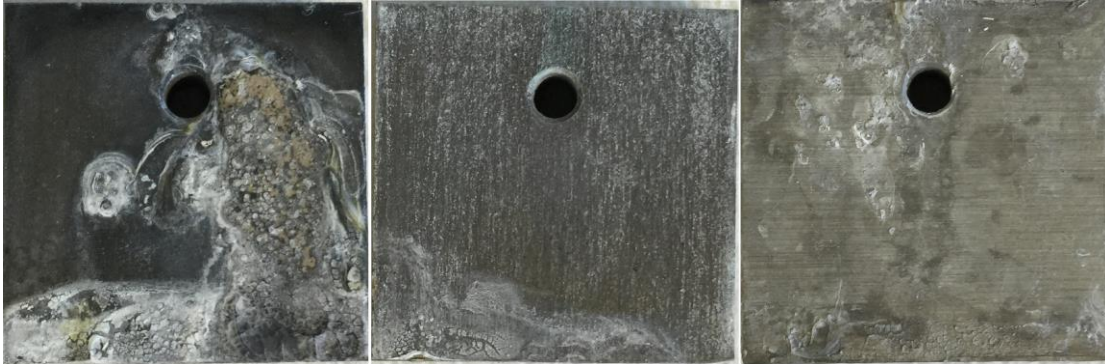
Figure 46. Corrosion Test Week 6, Left Superhydrophobic, Middle Superhydrophilic, Right Untreated.
