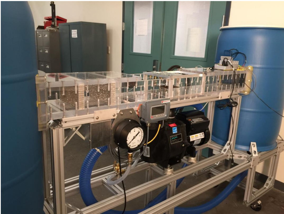
Figure 24. Assembled Testing Stand and Water Channel.
