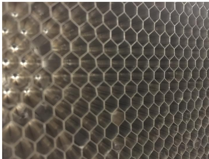
Figure 8. Sample of Hexagonal Honeycomb Flow Conditioner.
