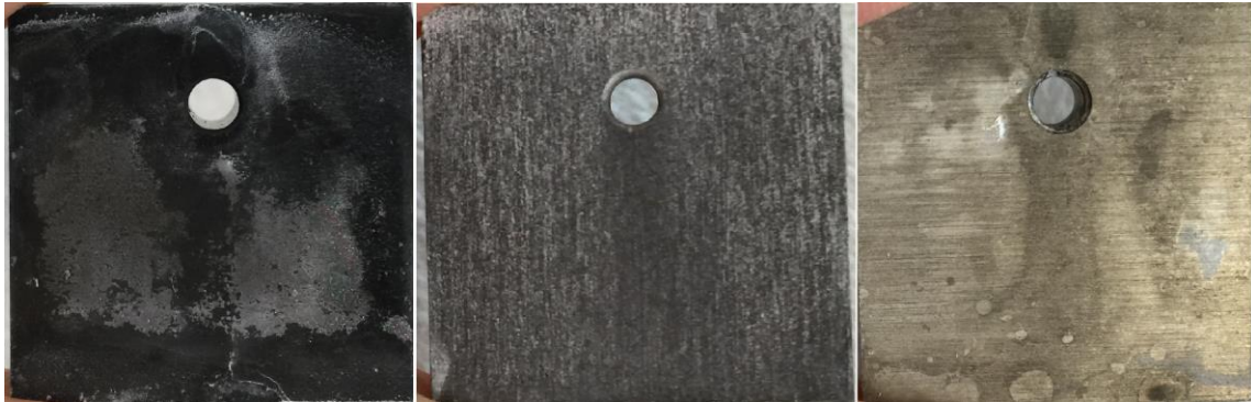
Figure 41. Corrosion Test Week 2, Left Superhydrophobic, Middle Superhydrophilic, Right Untreated.
