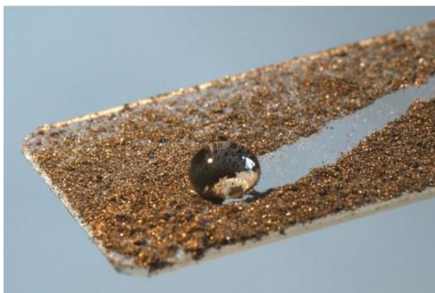
Figure 1. Self-Cleaning Action on a Superhydrophobic Surface. Source: [6]
