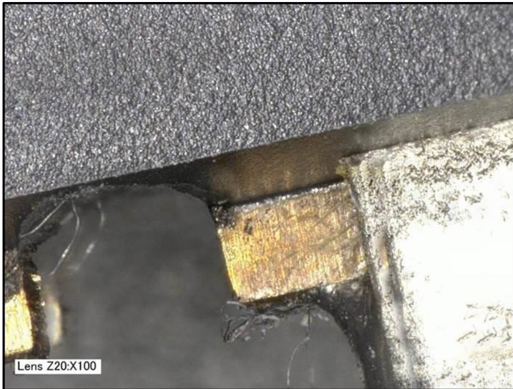
Figure 8-3: Metallic Whiskers (courtesy 3M)
