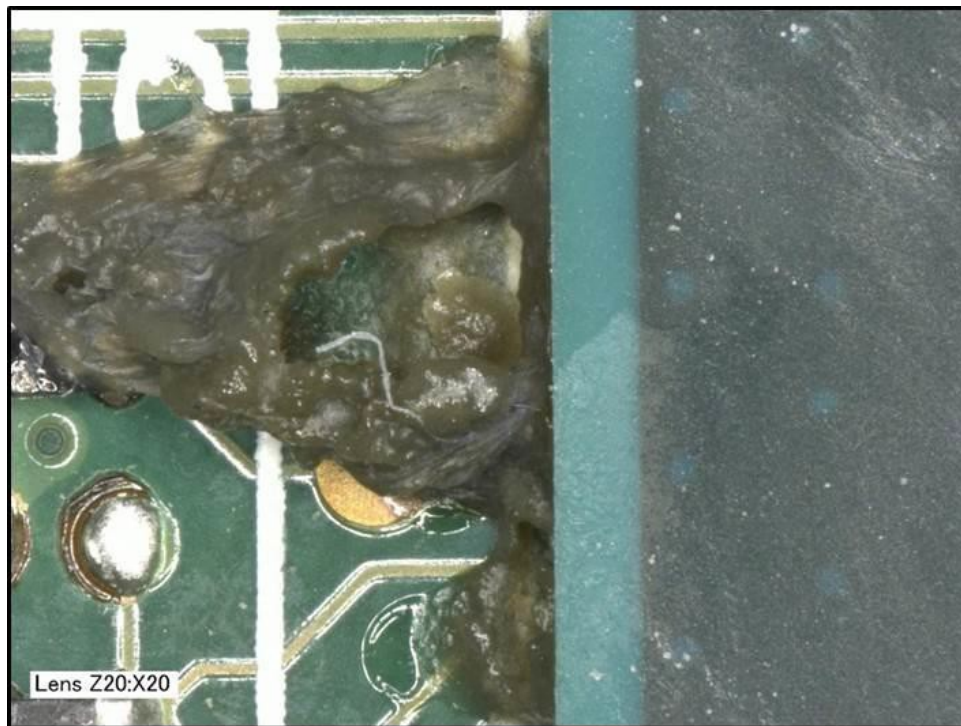
Figure 8-2: “Goop” With Whisker (courtesy of 3M)
