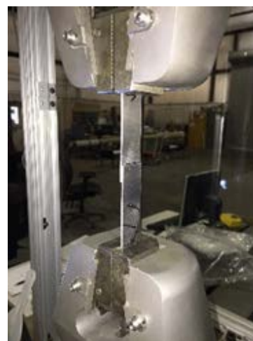
Figure 6. Lap shear specimen in Instron
