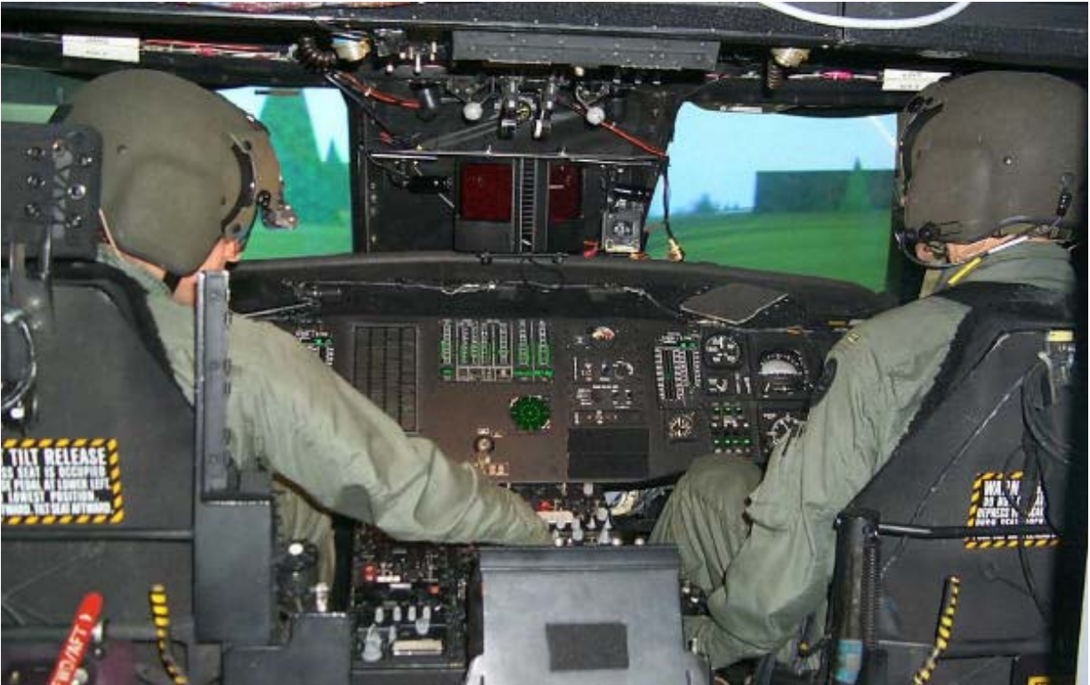
Figure 1. Cockpit of the U.S. Army Aeromedical Research Laboratory NUH-60FS Black Hawk Flight Simulator.
