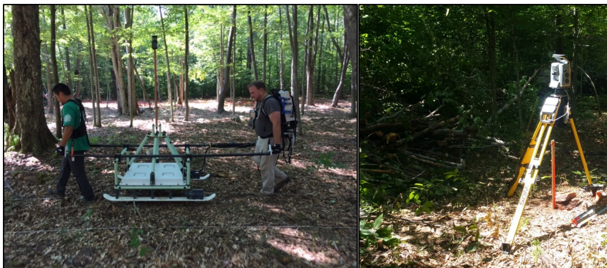
Figure 2-4. TOAR Survey Area Conditions, TEMTADS with MT1000 Prism, and RTK Base Station
