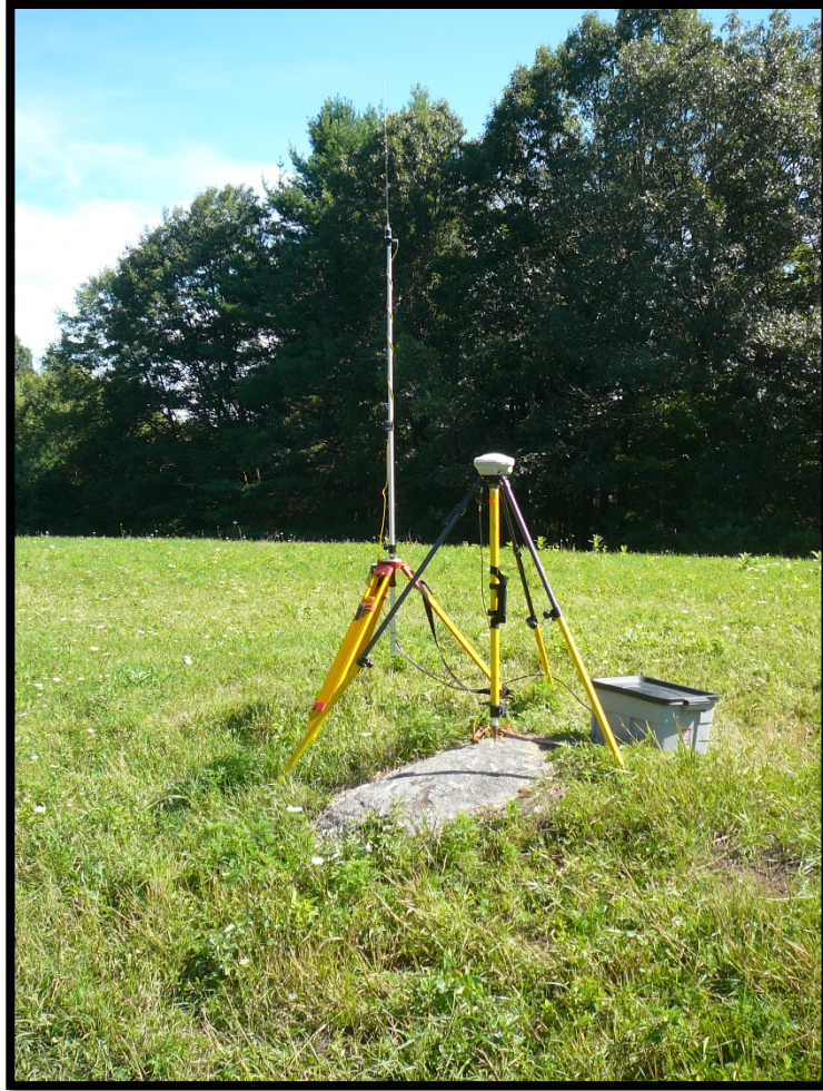
Figure 2-3. NBAFS RTK GPS Base Station
