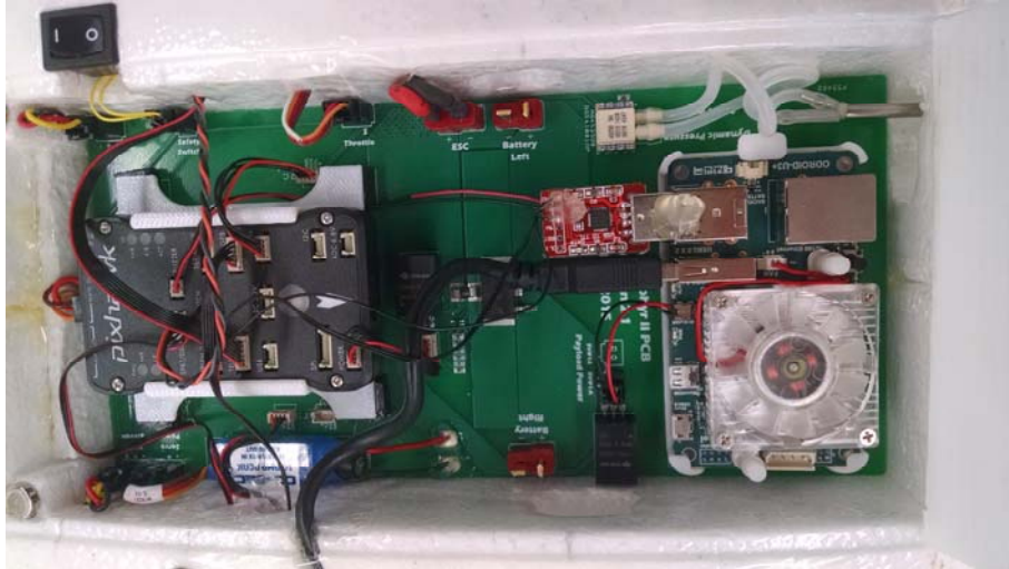
Figure 4. NPS UAV Motherboard Including ODroid
