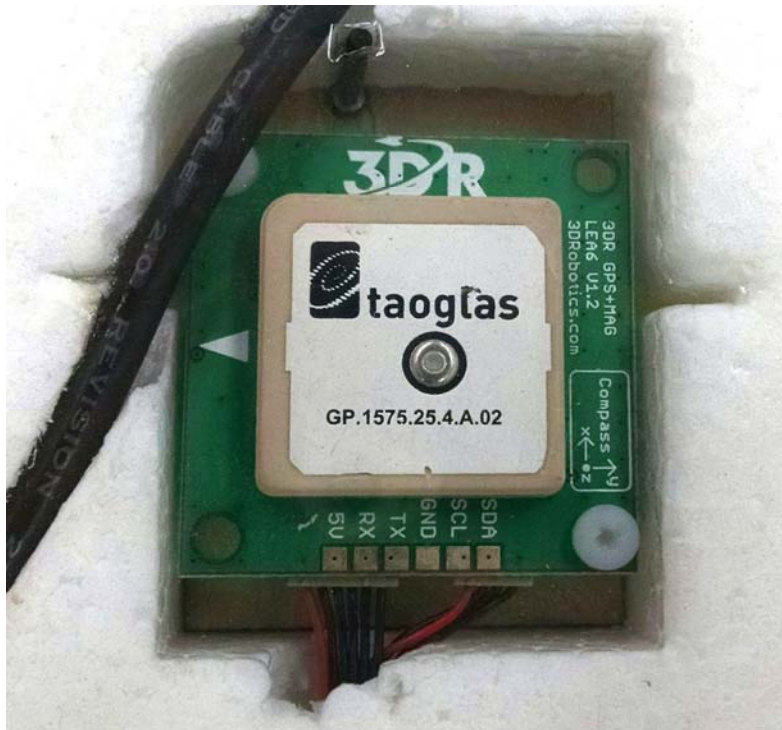
Figure 3. Picture of the GPS and Magnetic Sensor on the NPS UAV
