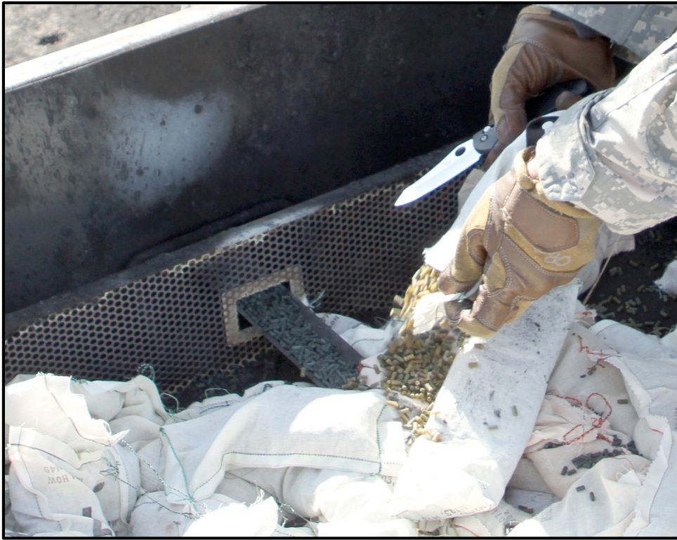
Figure 9: Placing propellant grains at the end of the slider to initiate burn
