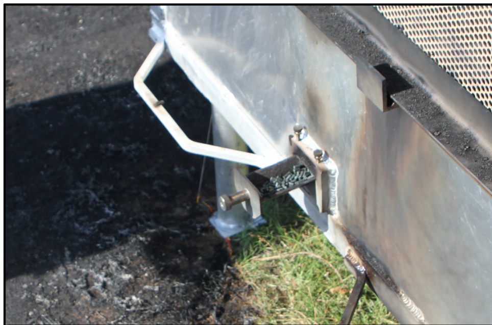
Figure 8: Propellant grains in ignition slider. Note the quantity of grains in slider.
