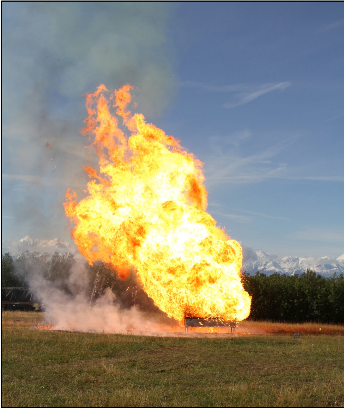
Figure 6: Howitzer propellant burn at \frac{3}{4} capacity. Note grass burning from radiant heat.
