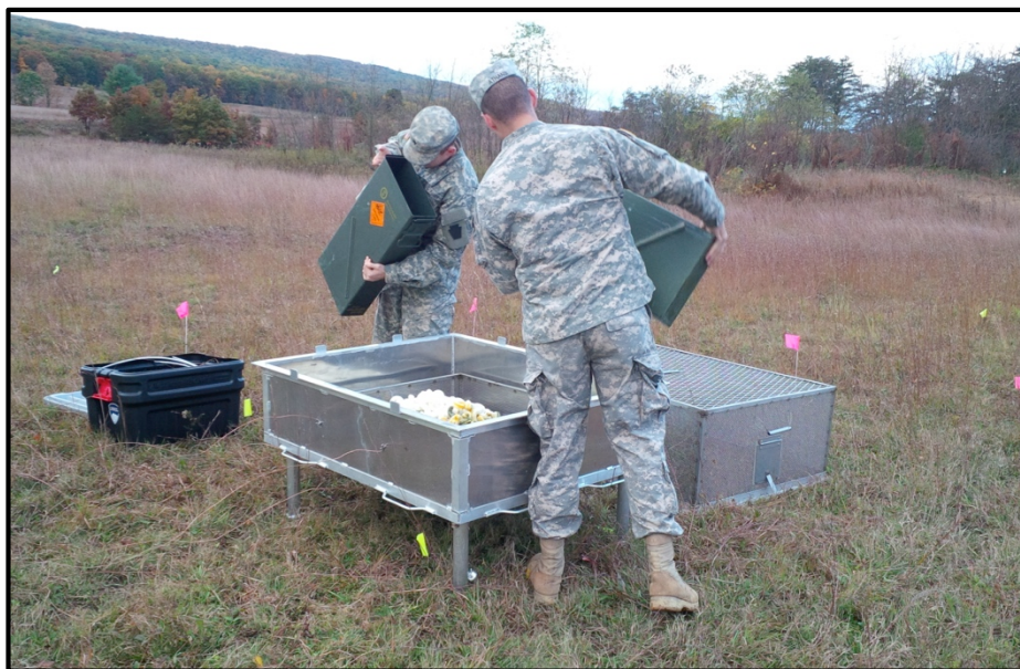
Figure 2: Mortar squad members loading excess propellant charges into a mortar training system burn pan. The bonnet is to the right of the pan.
