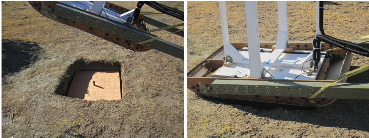
Figure 5. Library data collection. Library objects are placed in a clean area such as test pit (left). Once centered, the sensor head is lowered over the object for data collection (right).
