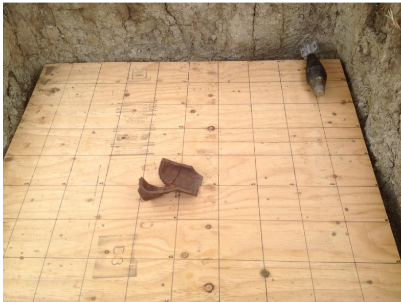
Figure 9. Test pit layout for multi-object scenario. The MetalMapper center was positioned over the frag item.
