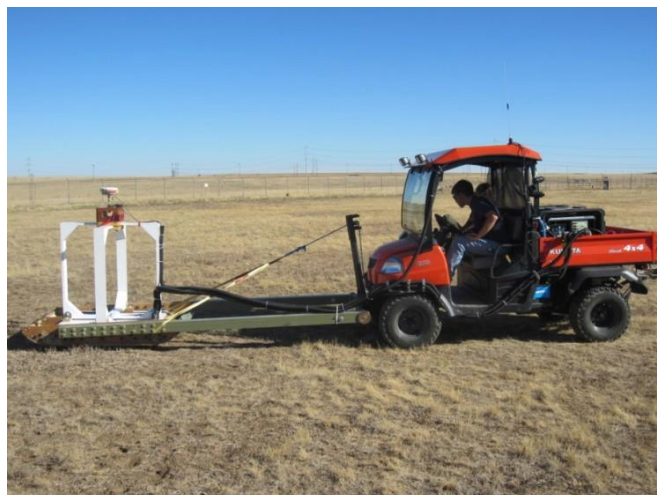
Figure 22. Mock cued survey performed at FLBGR compound. Target objects were placed near surveyed locations around the site.
