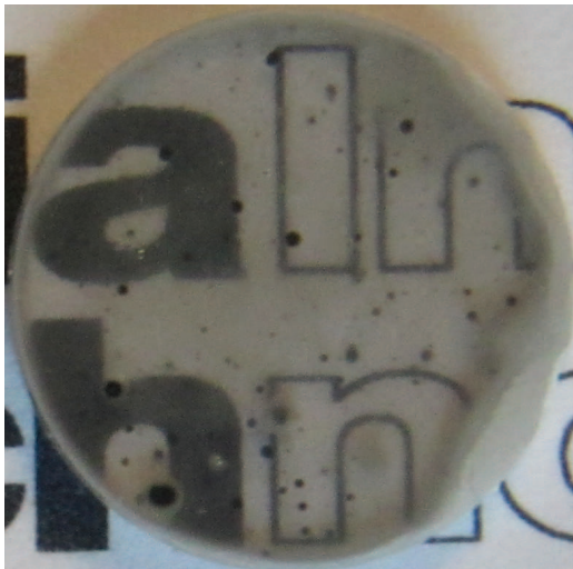
Figure 11: (left) Specimen sintered at 1600°C in the graphite heating-element furnace for 4 h and post-HIPed at 1600°C for 4 h, to a relative density of 99.60%.
