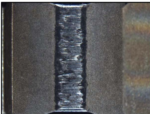
Figure 11. Bushing wear scar after testing for 2 h at 260°C and 333.6 N. The scar exhibits severe abrasive wear and is without the black lubricious transfer film.
