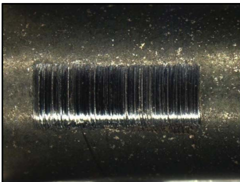
Figure 5. PS400 wear scar after testing at 760°C and 444.4 N. The scar exhibits a fully formed black oxide layer with light abrasive wear marks and polishing.
