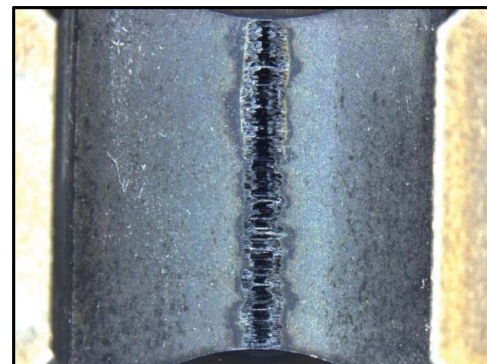
Figure 6. Bushing wear scar after testing at 760°C and 444.4 N. The wear scar exhibits light abrasive wear marks and polishing. The black film indicates a transfer of fluoride lubricants from the PS400.
