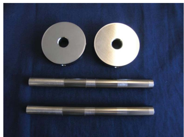
Figure 1. Bushing and rod test specimens. The three dark bands on the two rods are PS400.
