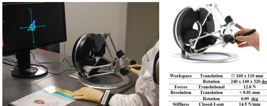
Figure 1. Shows the setup of the VR station during a data collection along with the six degree of freedom Omega device and its parameters.
