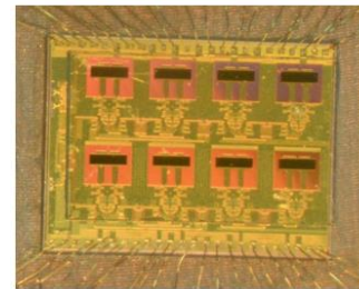
Fig.9: Schematic diagram and implemented structure for 94 GHz power amplifier / antenna array.
