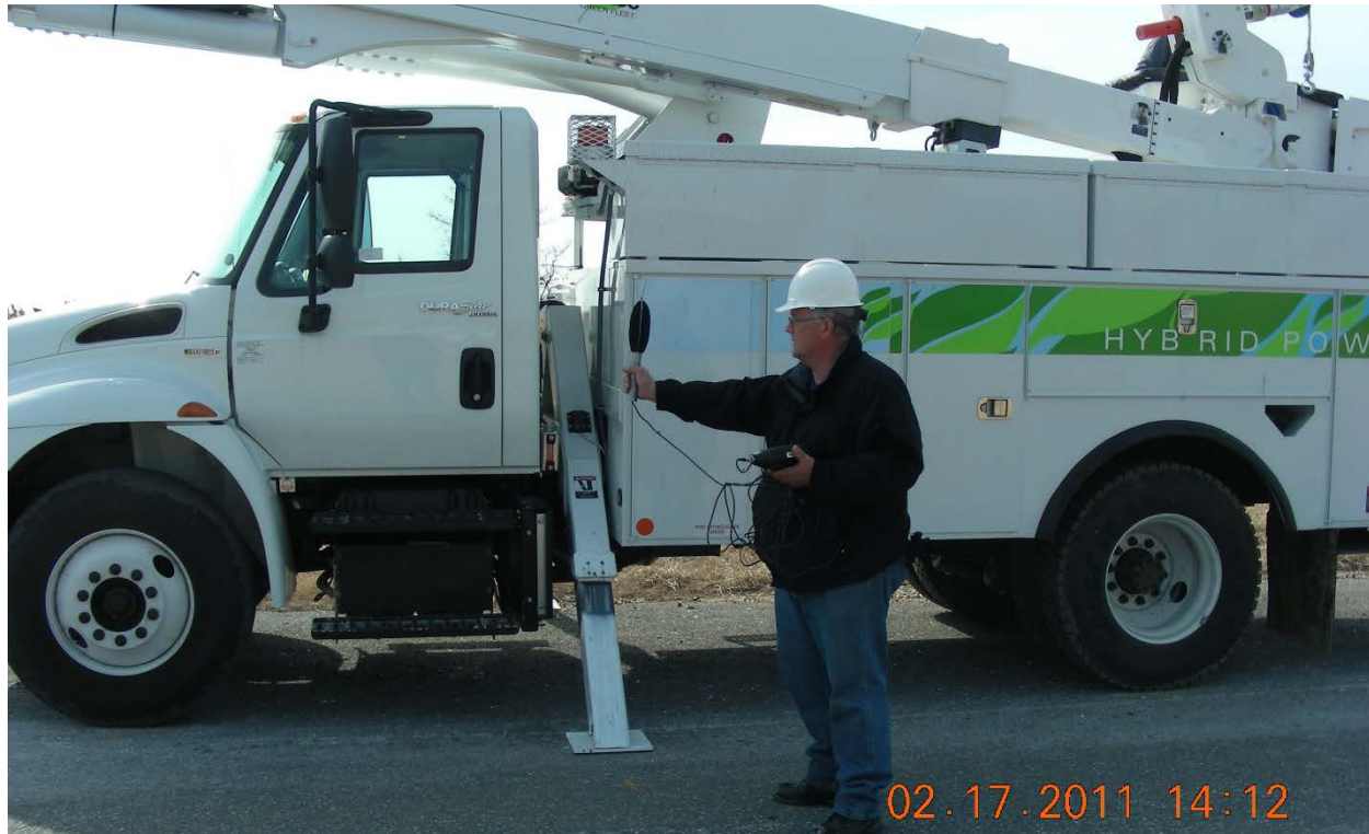
Figure 6-3. Photo of Personnel Collecting Perimeter Noise Measurements. (photo by Chris Shires, ATC)
